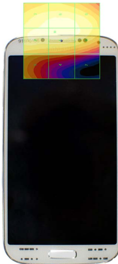
Figure 18-4 E-Field WD Scan overlay
