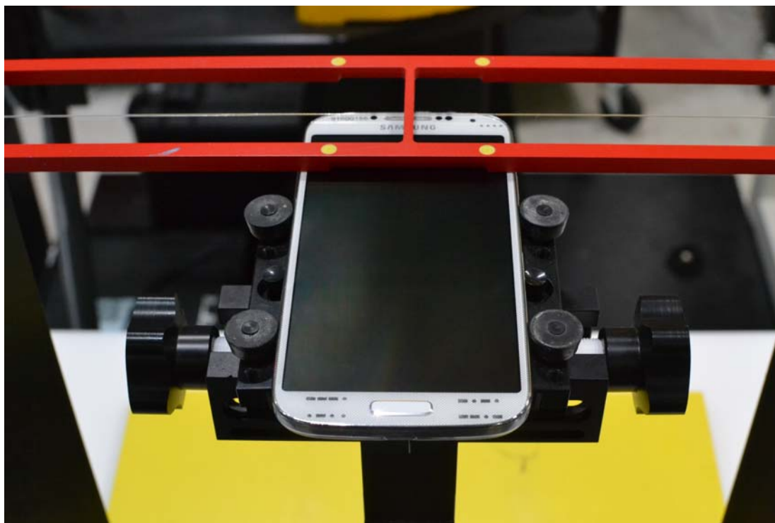
Figure 18-1 Ear Reference Point HAC Phantom Alignment
