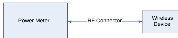
Figure 8-3 Power Measurement Setup
