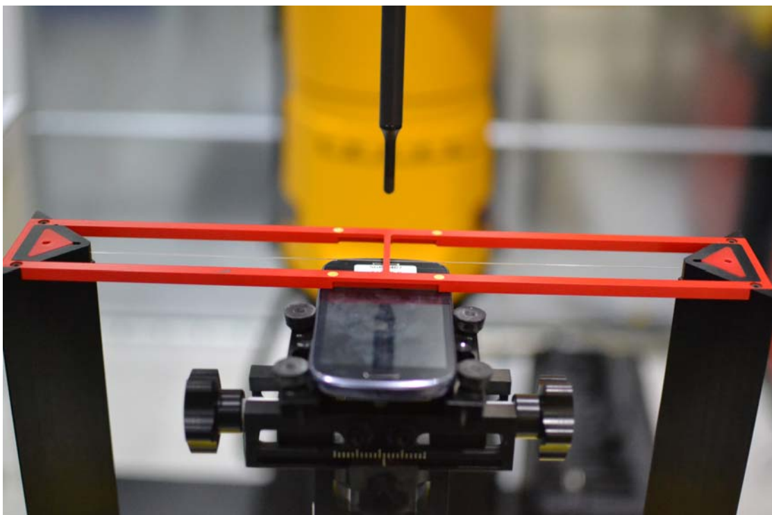
Figure 17-1 Ear Reference Point HAC Phantom Alignment
