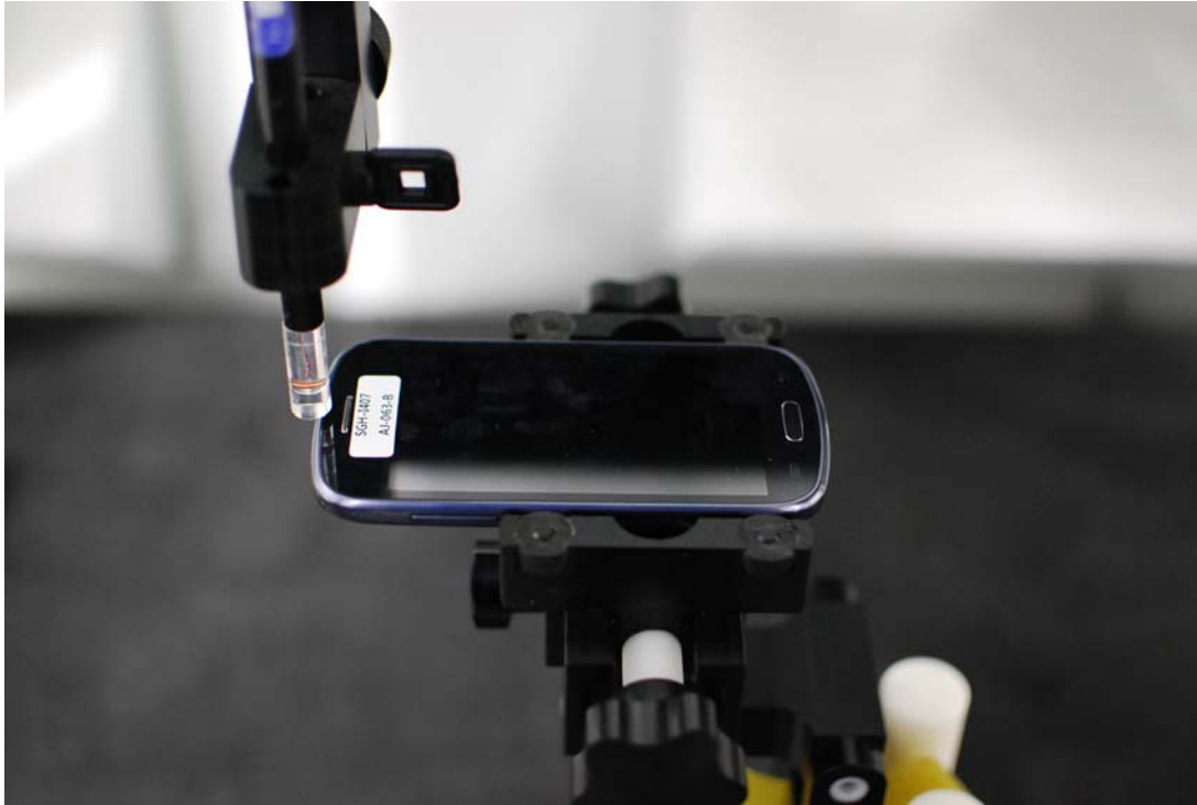
Figure 13-1 Test Setup for Wireless Device
