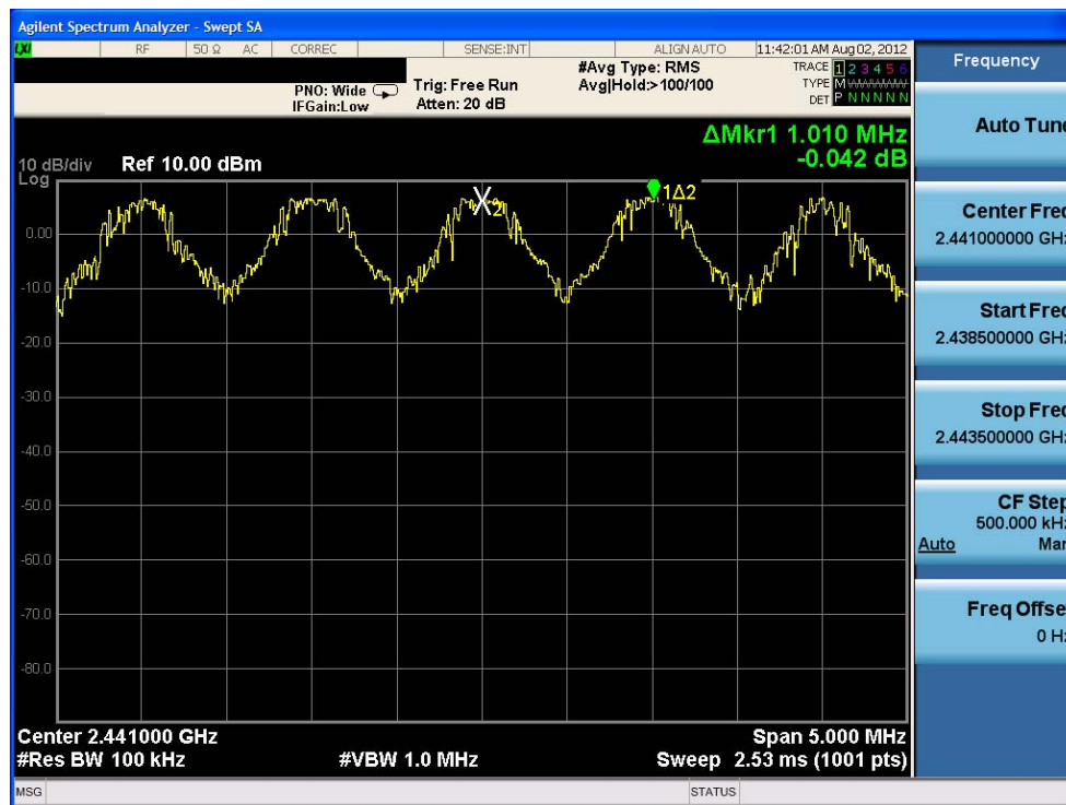
Plot 6-14. Channel Spacing Plot (Bluetooth)
