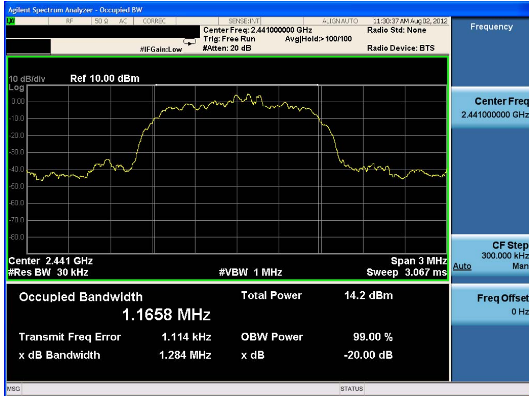
Plot 6-5. 20dB Bandwidth Plot (Bluetooth, 2Mbps – Ch. 39)
