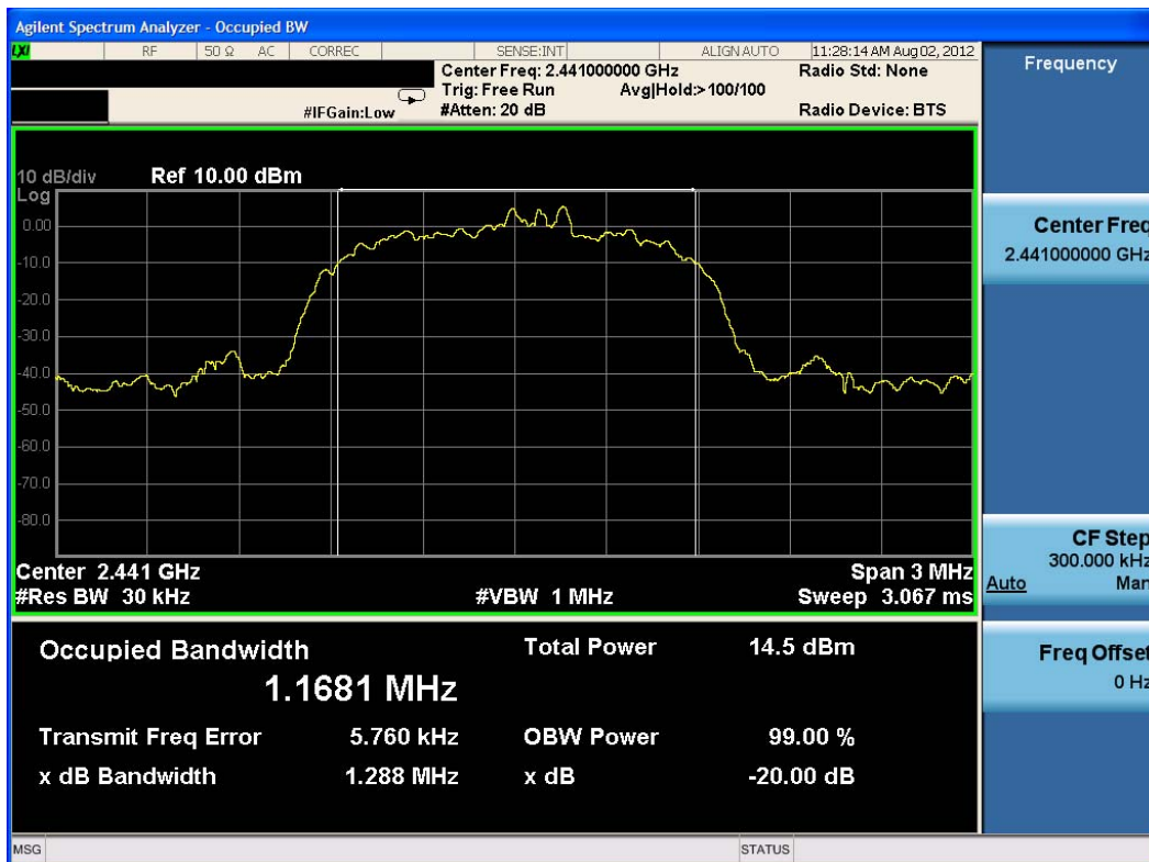
Plot 6-8. 20dB Bandwidth Plot (Bluetooth, 3Mbps – Ch. 39)
