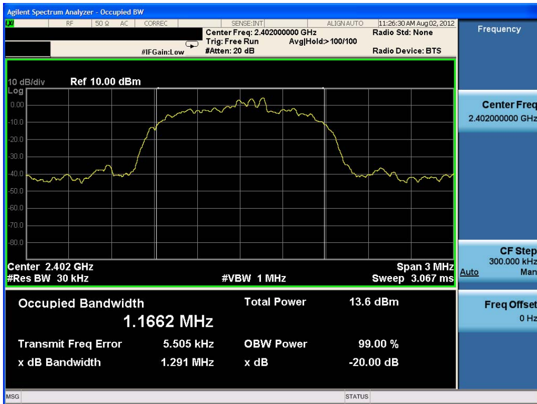
Plot 6-9. 20dB Bandwidth Plot (Bluetooth, 3Mbps – Ch. 78)
