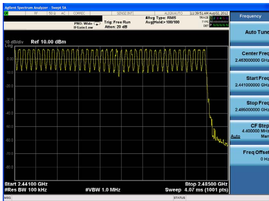
Plot 6-17. High End Spectrum Channel Hopping Plot (Bluetooth)
