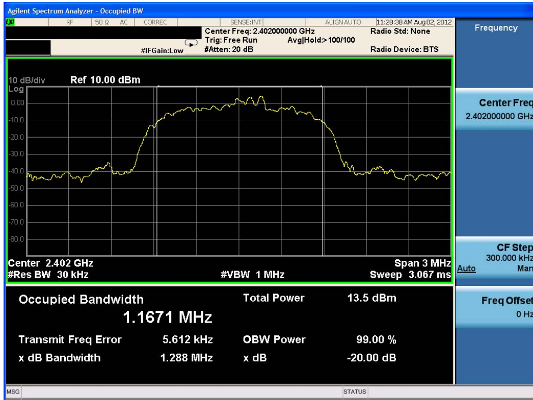
Plot 6-7. 20dB Bandwidth Plot (Bluetooth, 3Mbps – Ch. 0)
