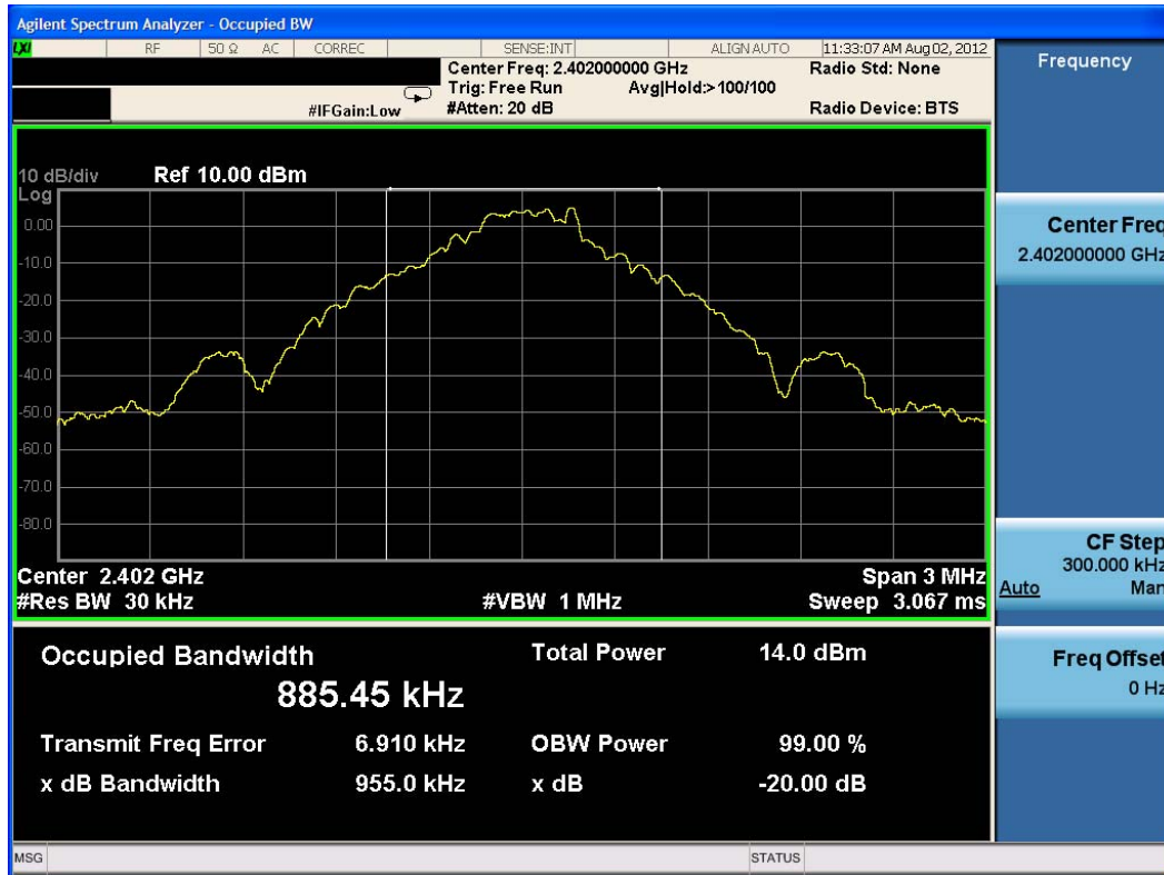
Plot 6-1. 20dB Bandwidth Plot (Bluetooth, 1Mbps – Ch. 0)
