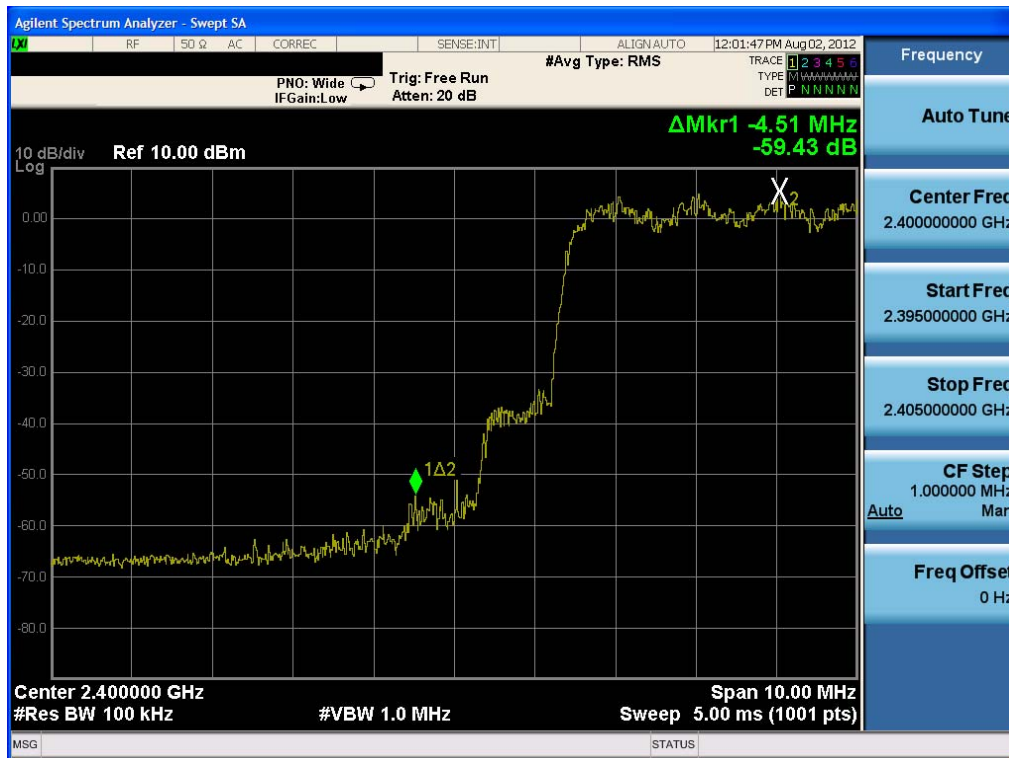
Plot 6-12. Band Edge Plot (Bluetooth with Hopping Enabled, 3Mbps)
