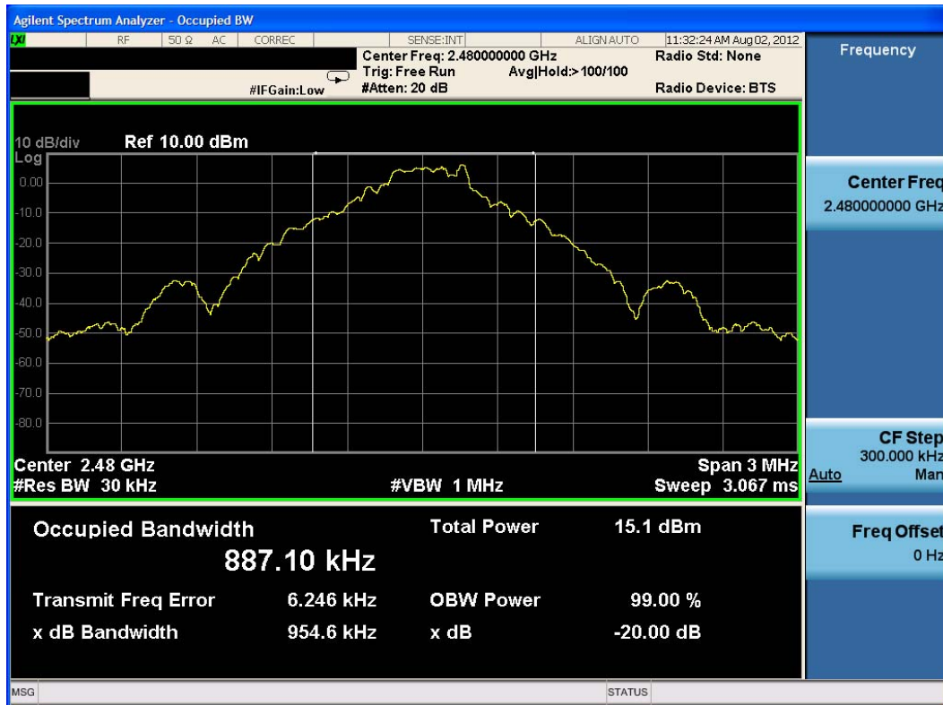
Plot 6-3. 20dB Bandwidth Plot (Bluetooth, 1Mbps – Ch. 78)
