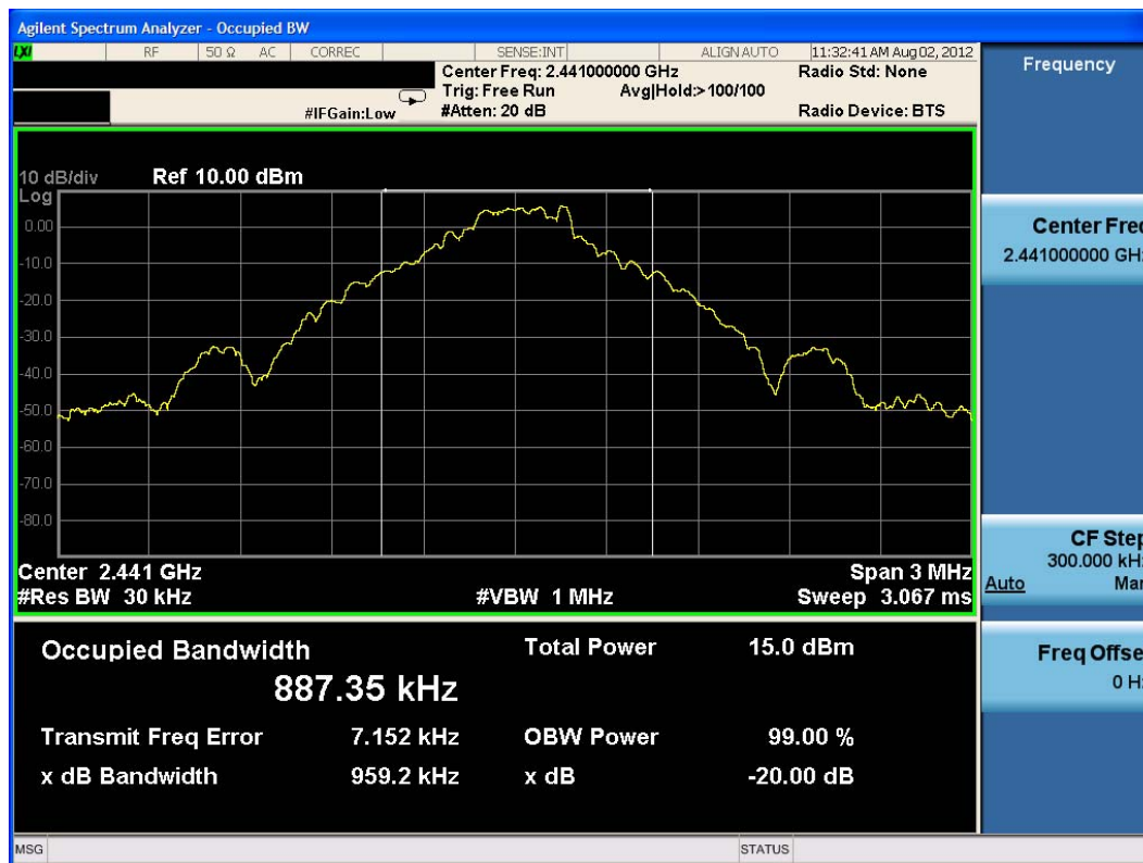
Plot 6-2. 20dB Bandwidth Plot (Bluetooth, 1Mbps – Ch. 39)
