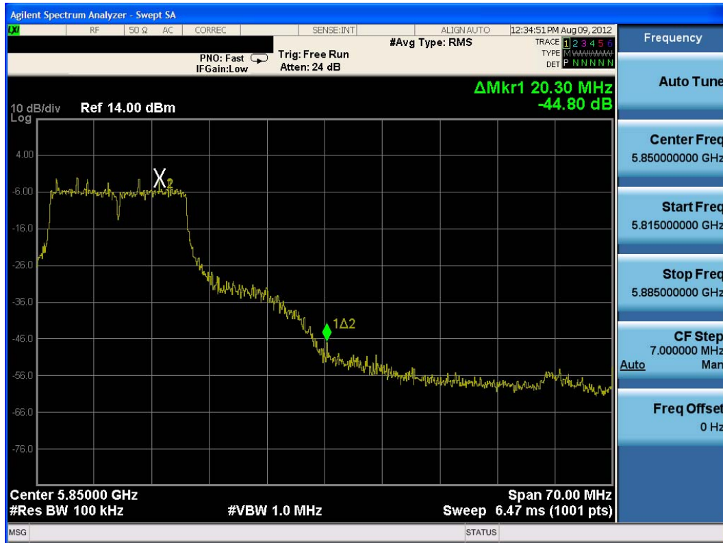
Plot 6-42. Band Edge Plot (802.11a – Ch. 165)
