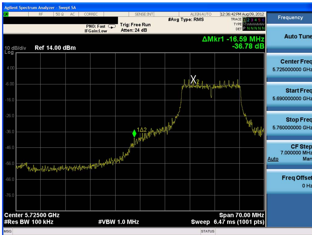
Plot 6-41. Band Edge Plot (802.11a – Ch. 149)
