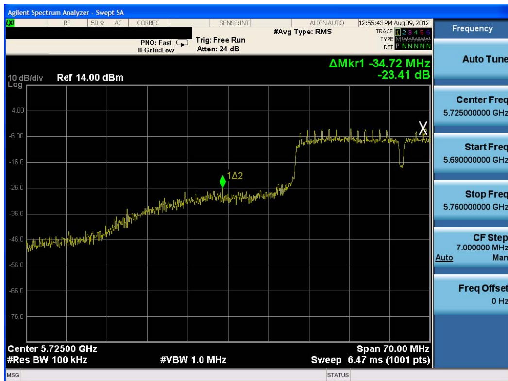
Plot 6-45. Band Edge Plot (40MHz BW 802.11n (5.8GHz) – Ch. 151)
