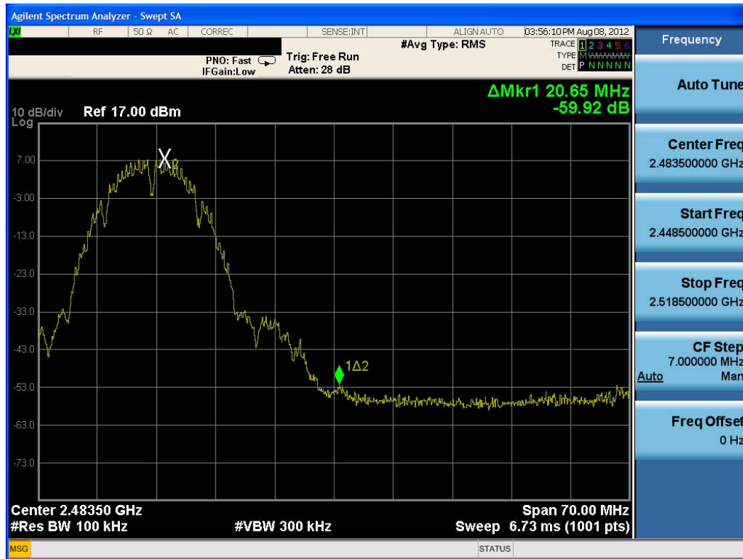
Plot 6-36. Band Edge Plot (802.11b – Ch. 11)
