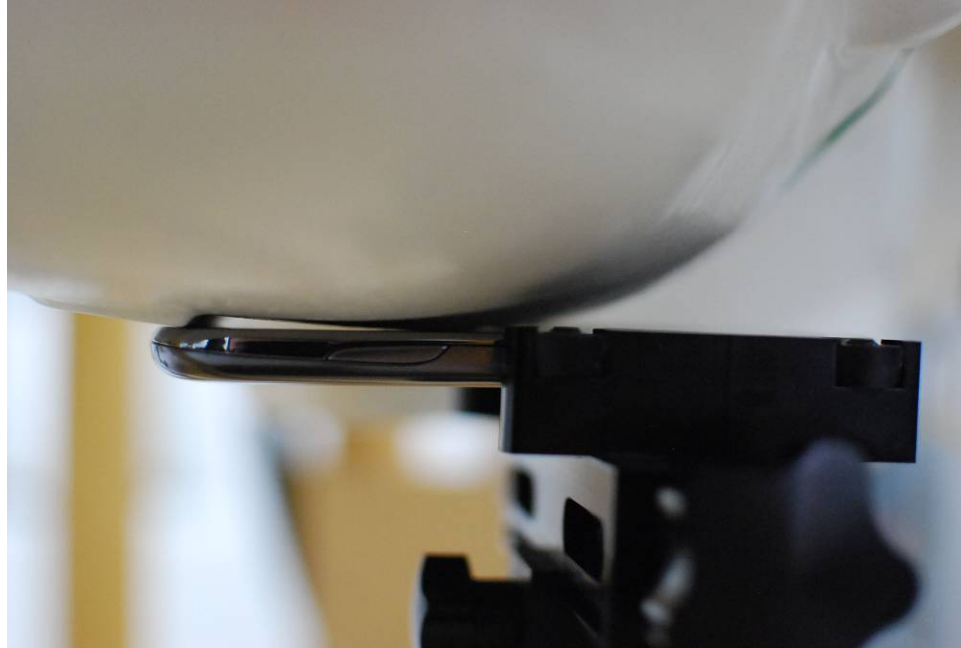
SAR Test Setup Photo 1 – Right Cheek
