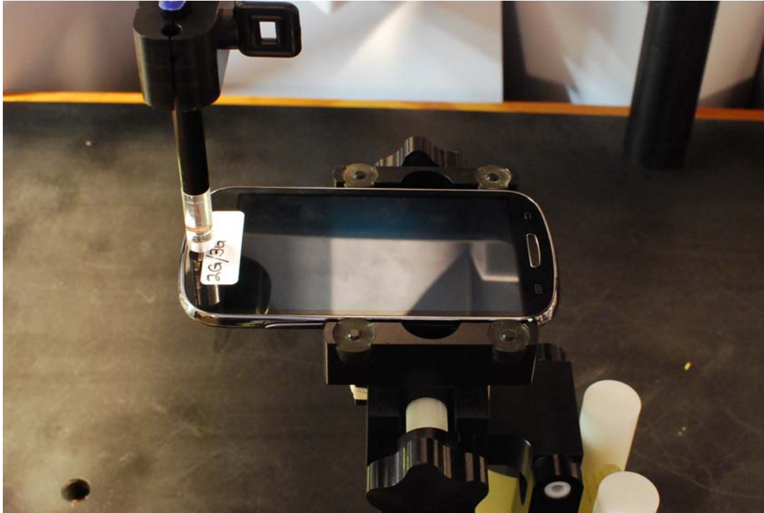
Figure 13-1 Test Setup for Wireless Device
