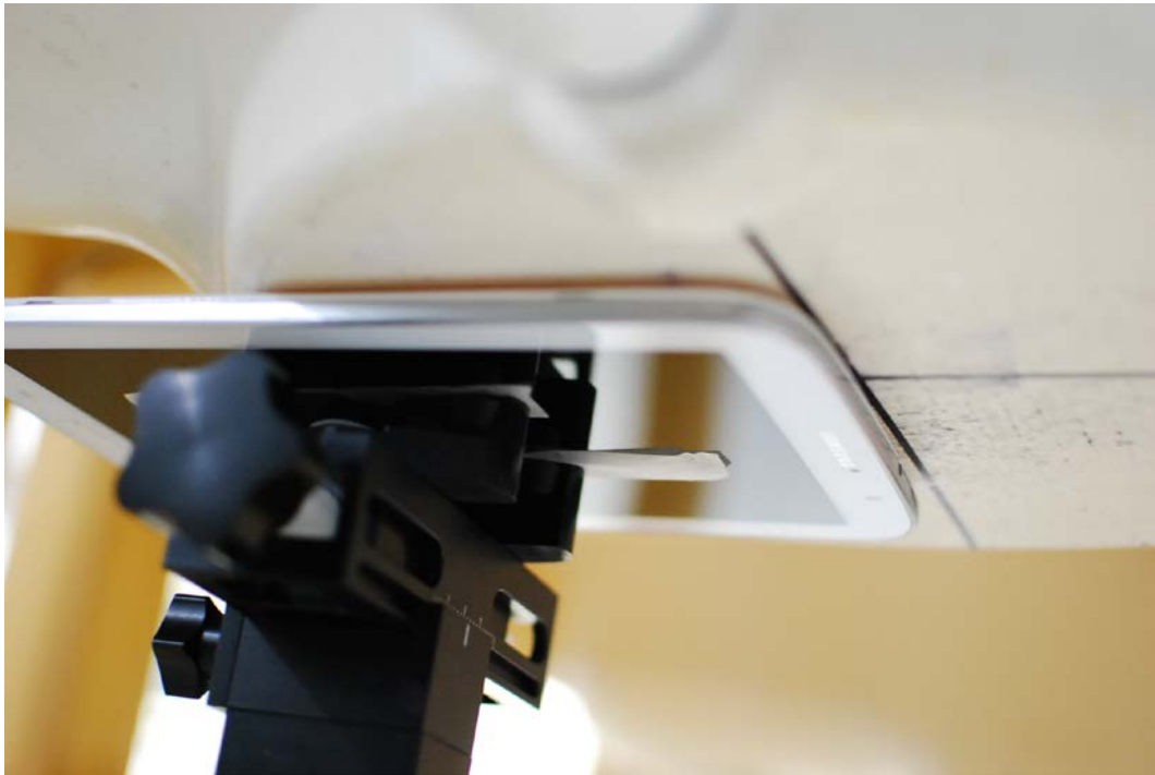
SAR Test Setup Photo 1: Back at 0.0 mm
