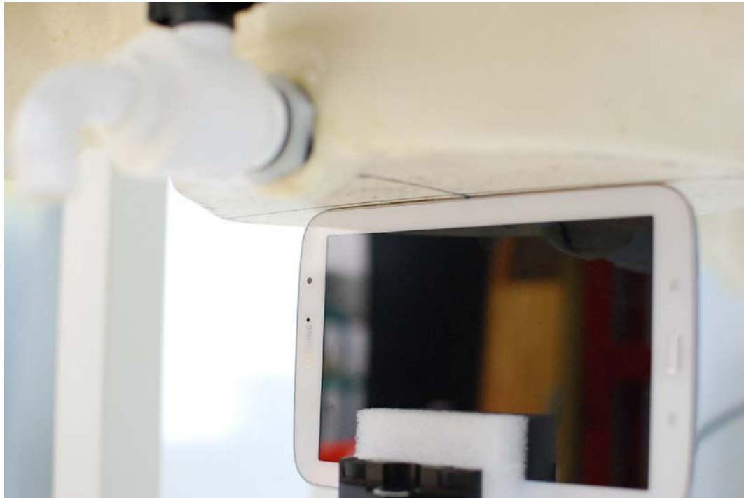
SAR Test Setup Photo 5: Right at 0 mm
