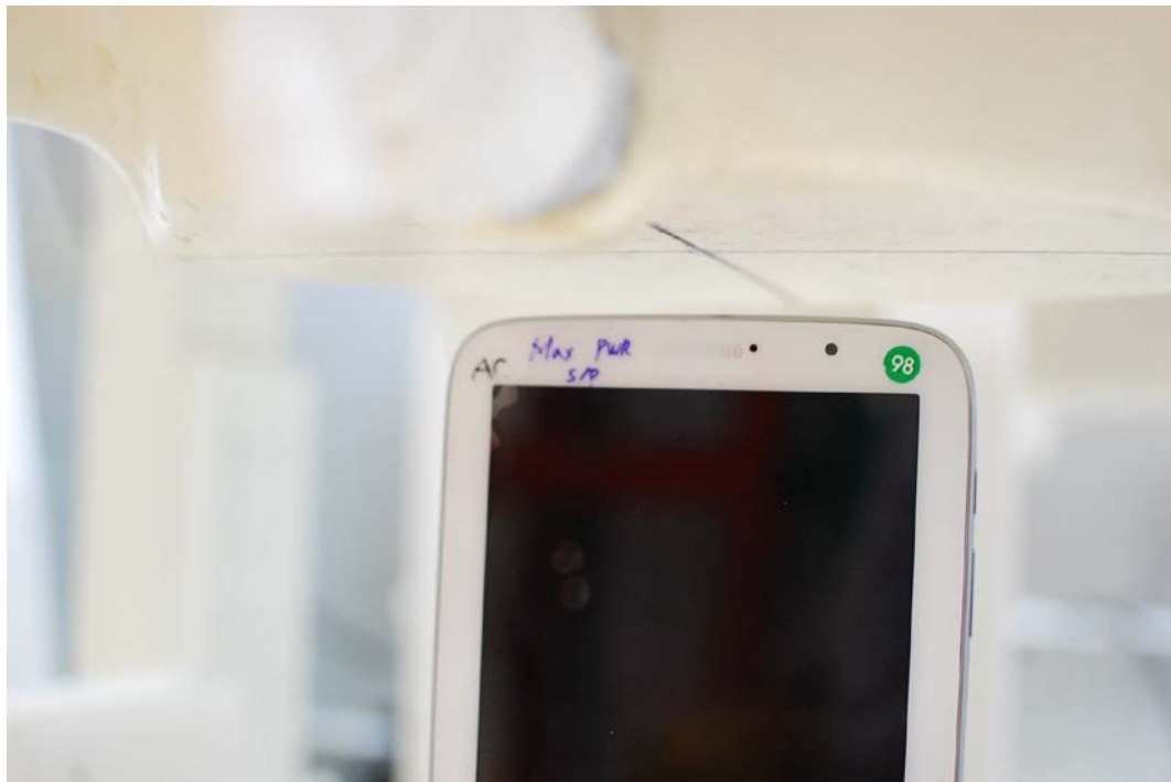
SAR Test Setup Photo 4: Top at 15 mm
