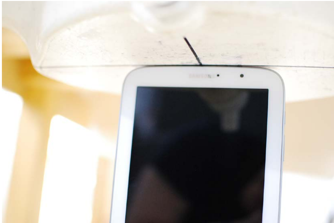
SAR Test Setup Photo 3: Top at 0.0 mm
