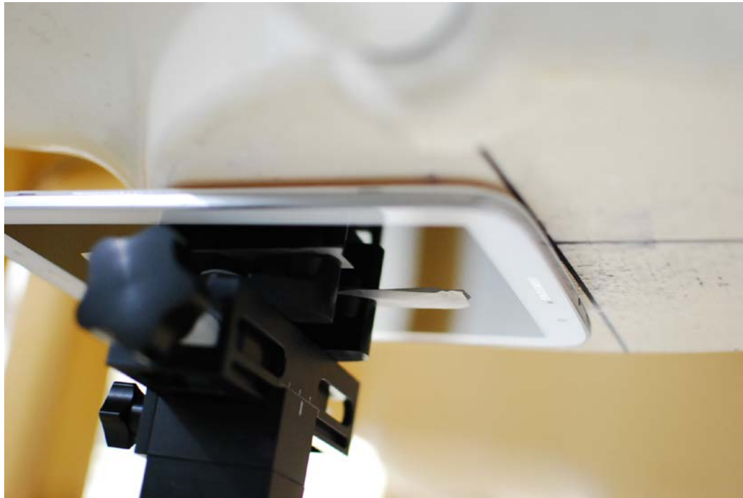
SAR Test Setup Photo 1: Back at 0.0 mm
