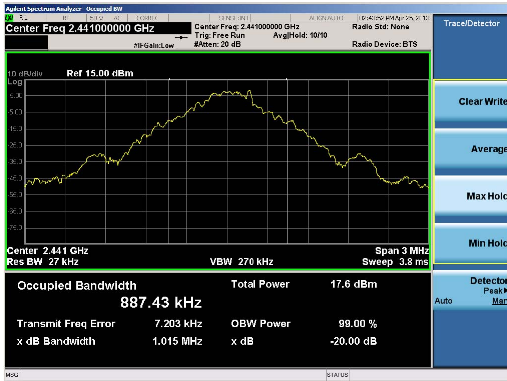
Plot 6-2. 20dB Bandwidth Plot (Bluetooth, 1Mbps – Ch. 39)
