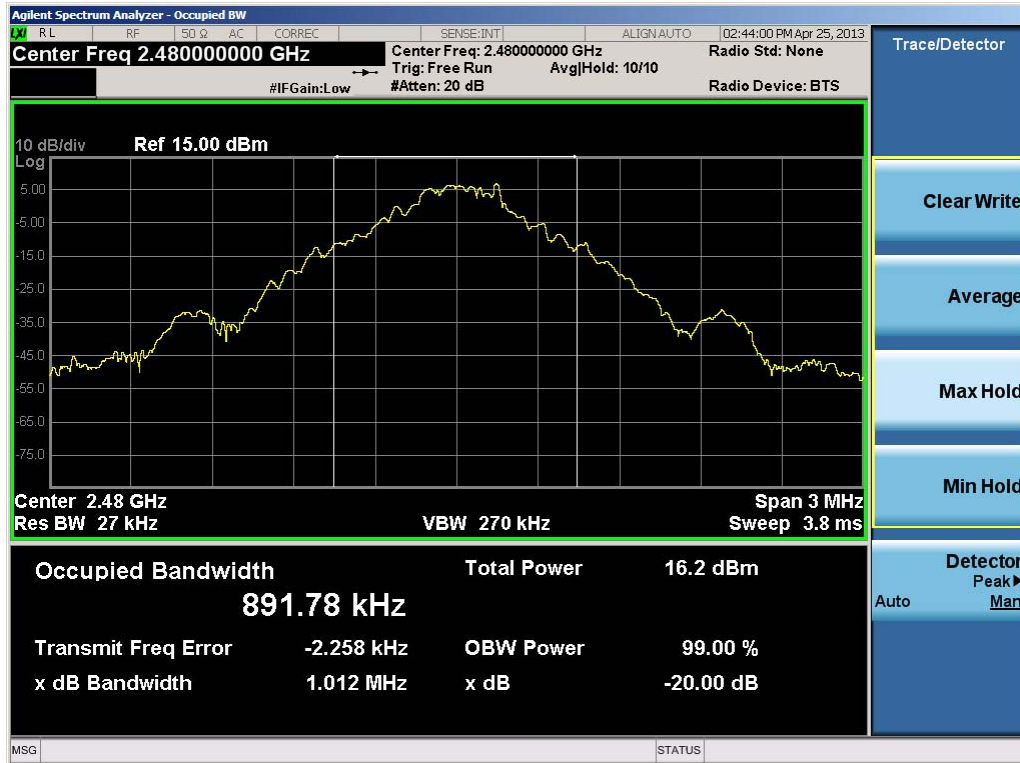
Plot 6-3. 20dB Bandwidth Plot (Bluetooth, 1Mbps – Ch. 78)
