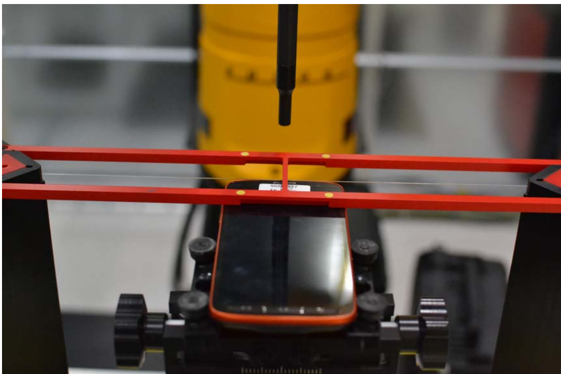
Figure 17-1 Ear Reference Point HAC Phantom Alignment
