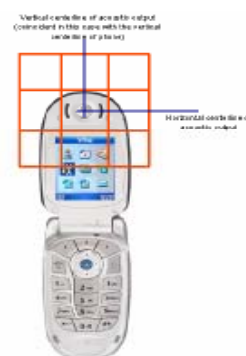
Figure 5.1 Wireless Device and Measurement Plane
