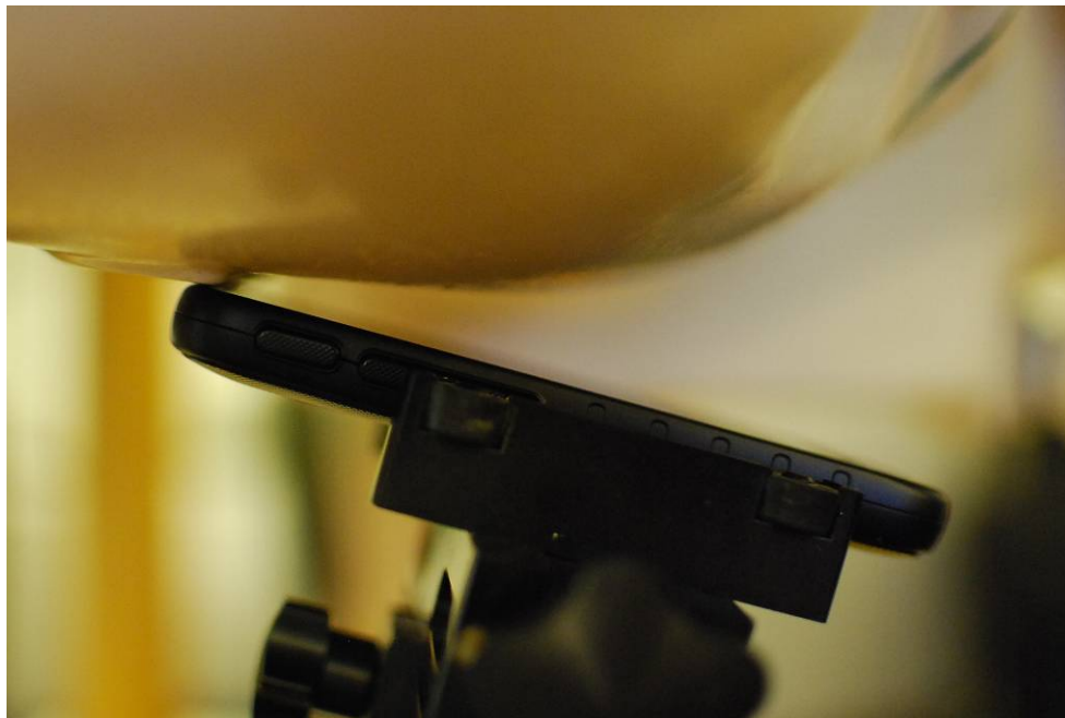
SAR Test Setup Photo 2: Right Tilt
