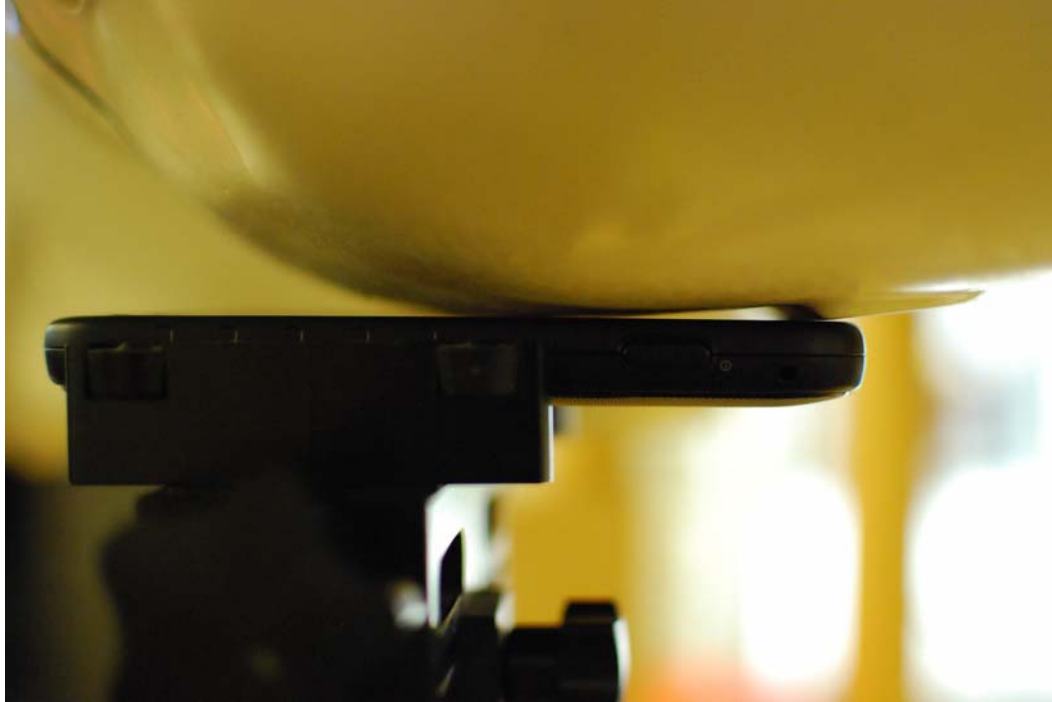
SAR Test Setup Photo 3: Left Touch
