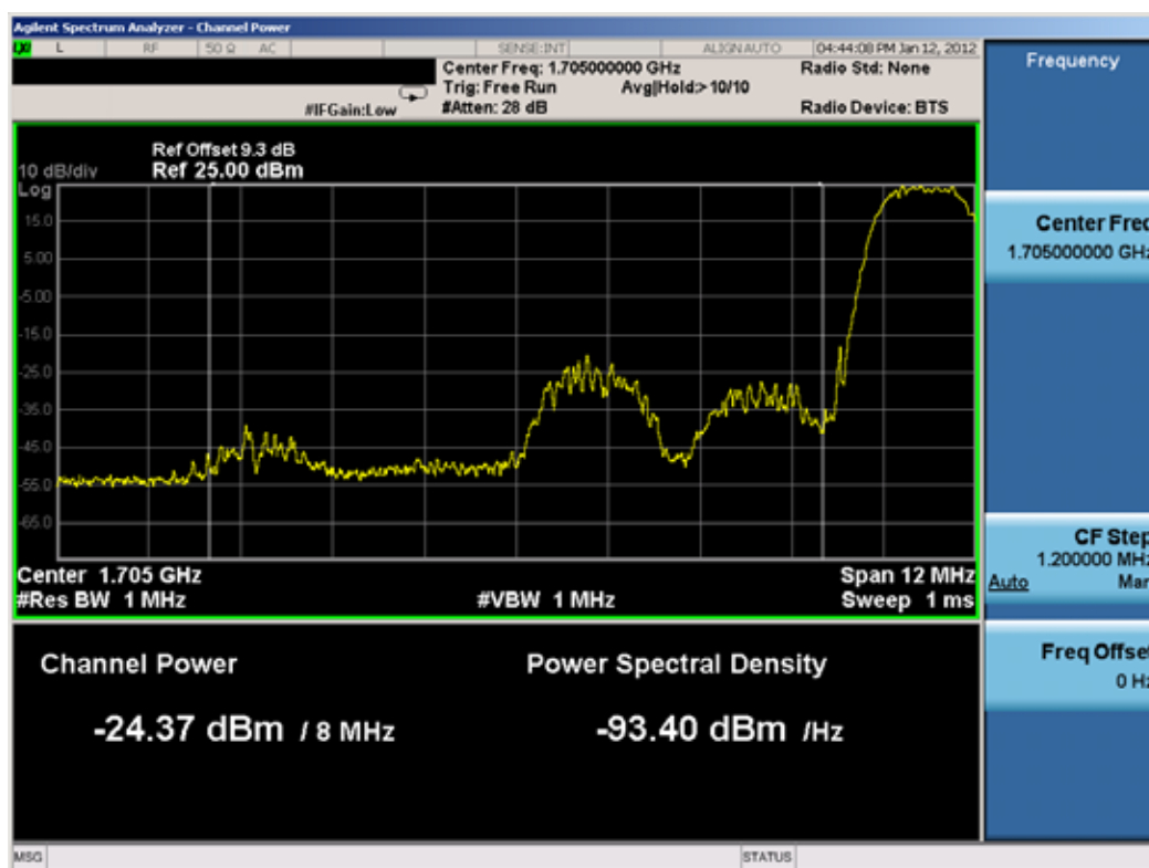
Plot 8-13. Extended Band Edge Plot (5MHz BW, QPSK RB Size = 1 Offset = 0)
