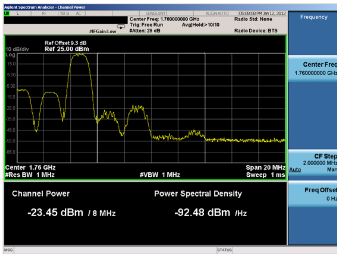
Plot 8-30. Extended Band Edge Plot (5MHz BW, QPSK RB Size = 1 Offset = 24, High Channel)
