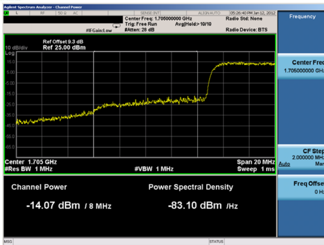
Plot 8-12. Extended Band Edge Plot (10MHz BW, QPSK RB Size = 50 Offset = 0)
