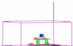
Figure 3-1. Shielded Enclosure Line-Conducted Test Facility
