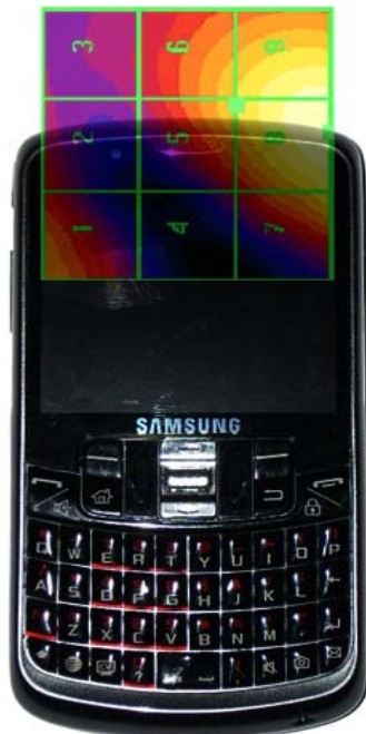
Figure 17-4 E-Field WD Scan overlay
