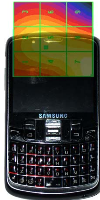
Figure 17-5 H-Field WD Scan overlay
