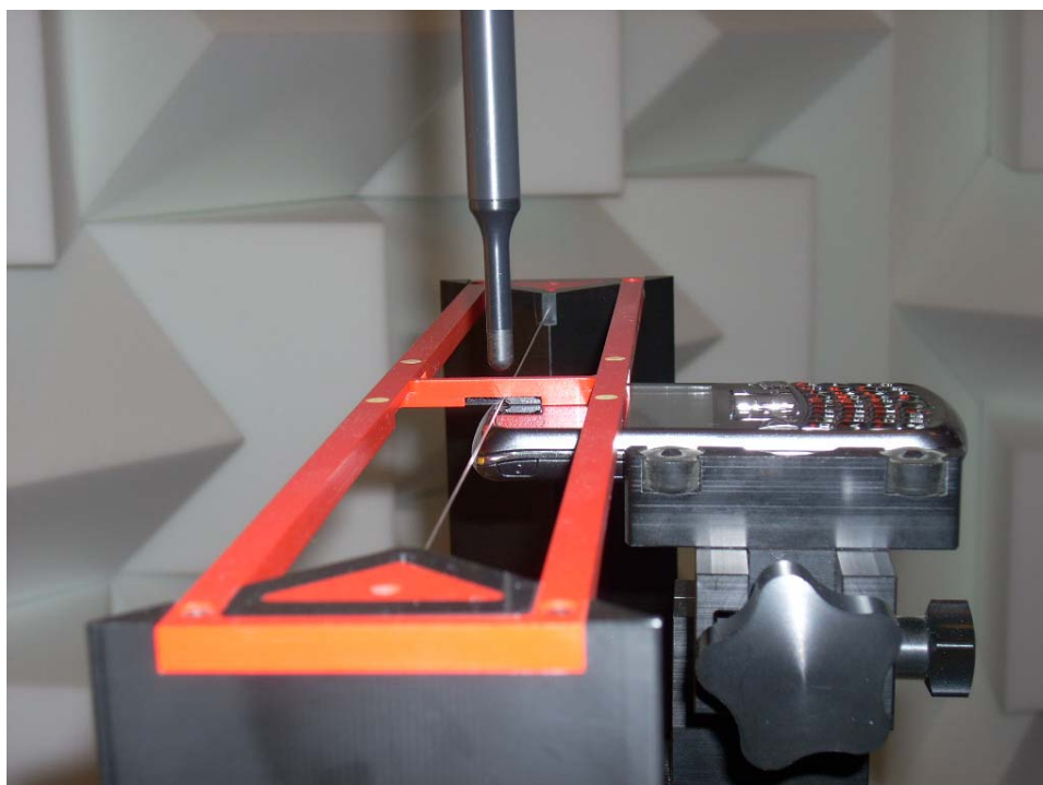
Figure 17-2 HAC Phantom Plane Alignment
