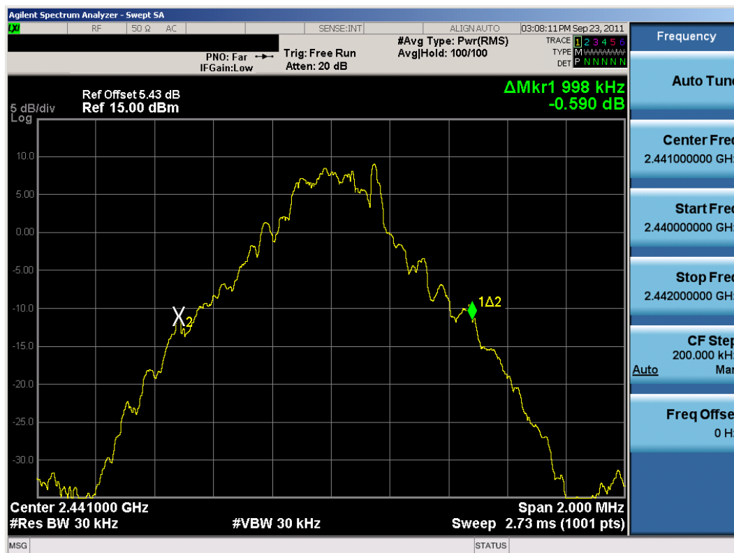
Plot 6-2. 20dB Bandwidth Plot (Bluetooth, 1Mbps – Ch. 39)
