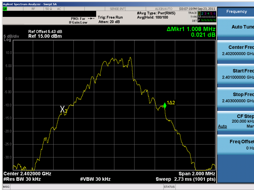
Plot 6-1. 20dB Bandwidth Plot (Bluetooth, 1Mbps – Ch. 0)
