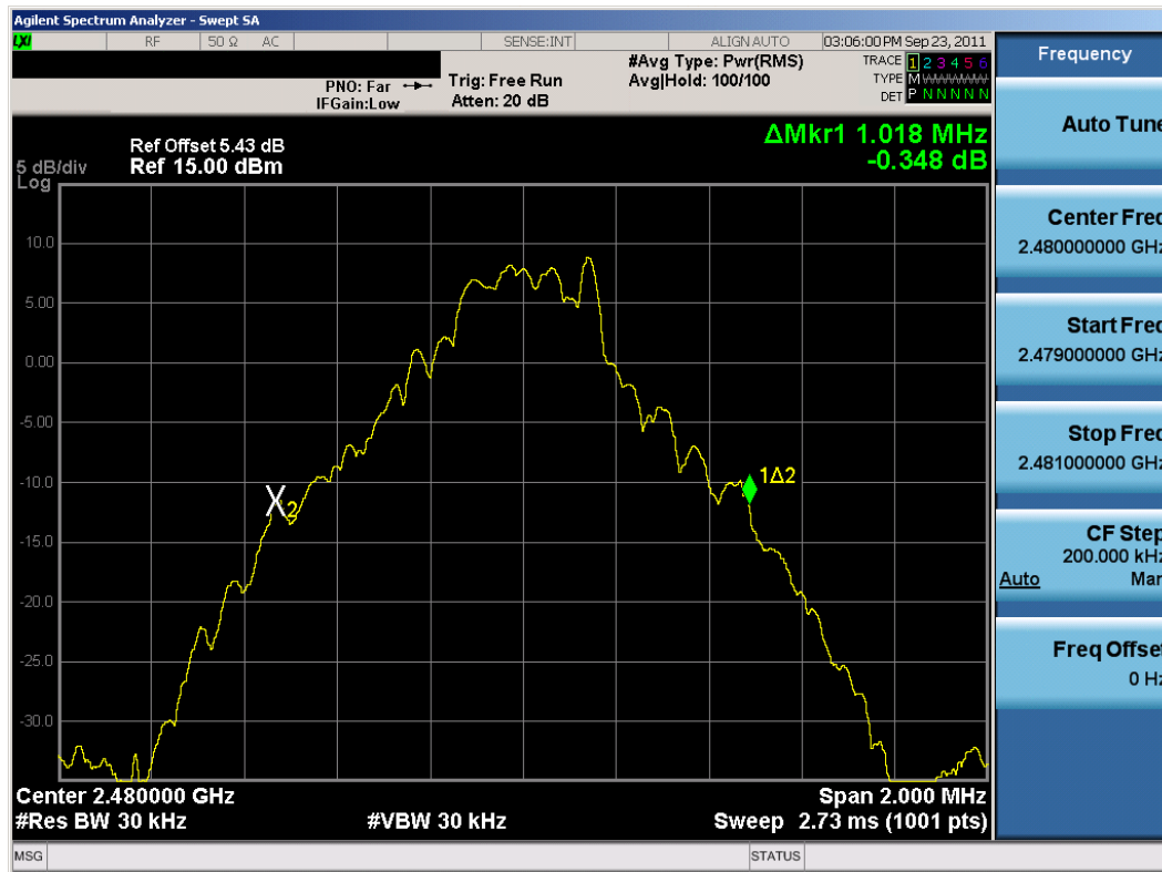
Plot 6-3. 20dB Bandwidth Plot (Bluetooth, 1Mbps – Ch. 78)
