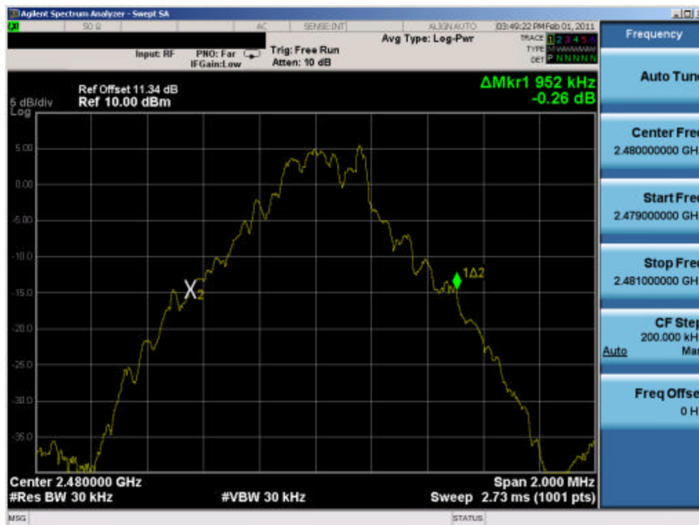
Plot 6-3. 20dB Bandwidth Plot (Bluetooth, 1Mbps – Ch. 78)
