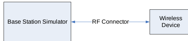
Figure 13-1 Power Measurement Setup
