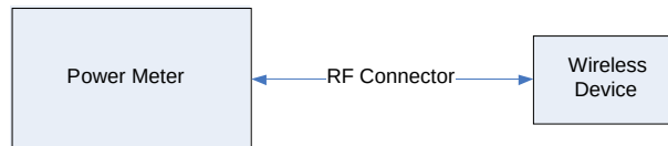
Figure 13-2 Power Measurement Setup
