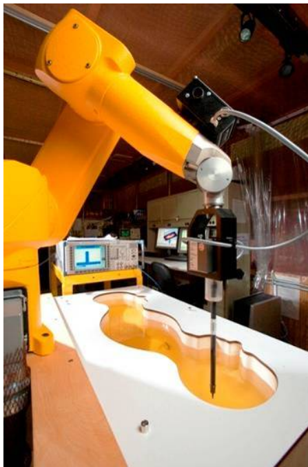
Figure 5-2 SAR Measurement System
