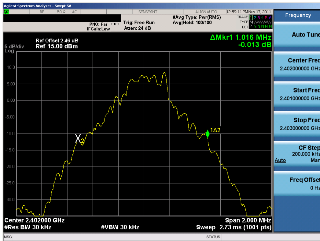
Plot 6-1. 20dB Bandwidth Plot (Bluetooth, 1Mbps - Ch. 0)
