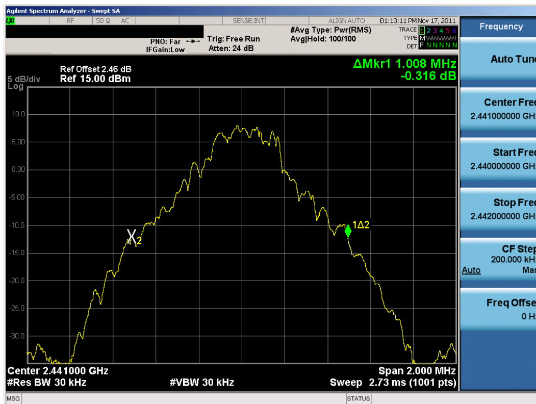
Plot 6-2. 20dB Bandwidth Plot (Bluetooth, 1Mbps - Ch. 39)
