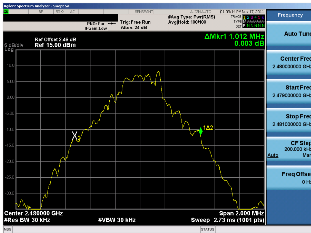
Plot 6-3. 20dB Bandwidth Plot (Bluetooth, 1Mbps – Ch. 78)
