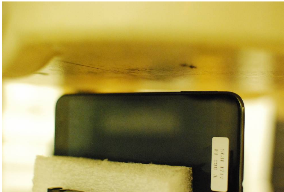
SAR Test Setup Photo 10: Left at 1.0 cm
