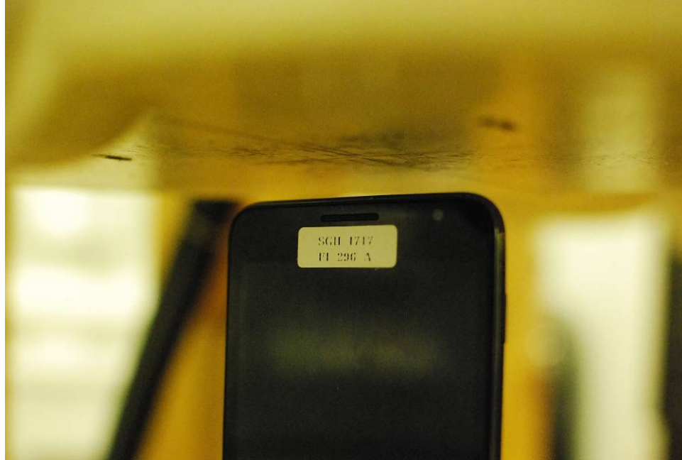
SAR Test Setup Photo 7: Top at 1.0 cm
