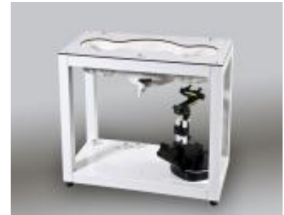
Figure 6-1 Twin SAM SAR Phantom
