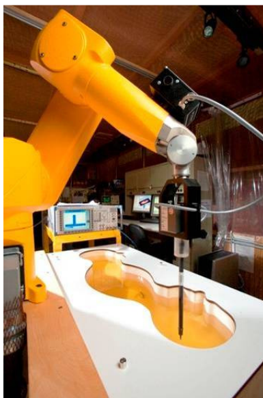
Figure 4-2 SAR Measurement System
