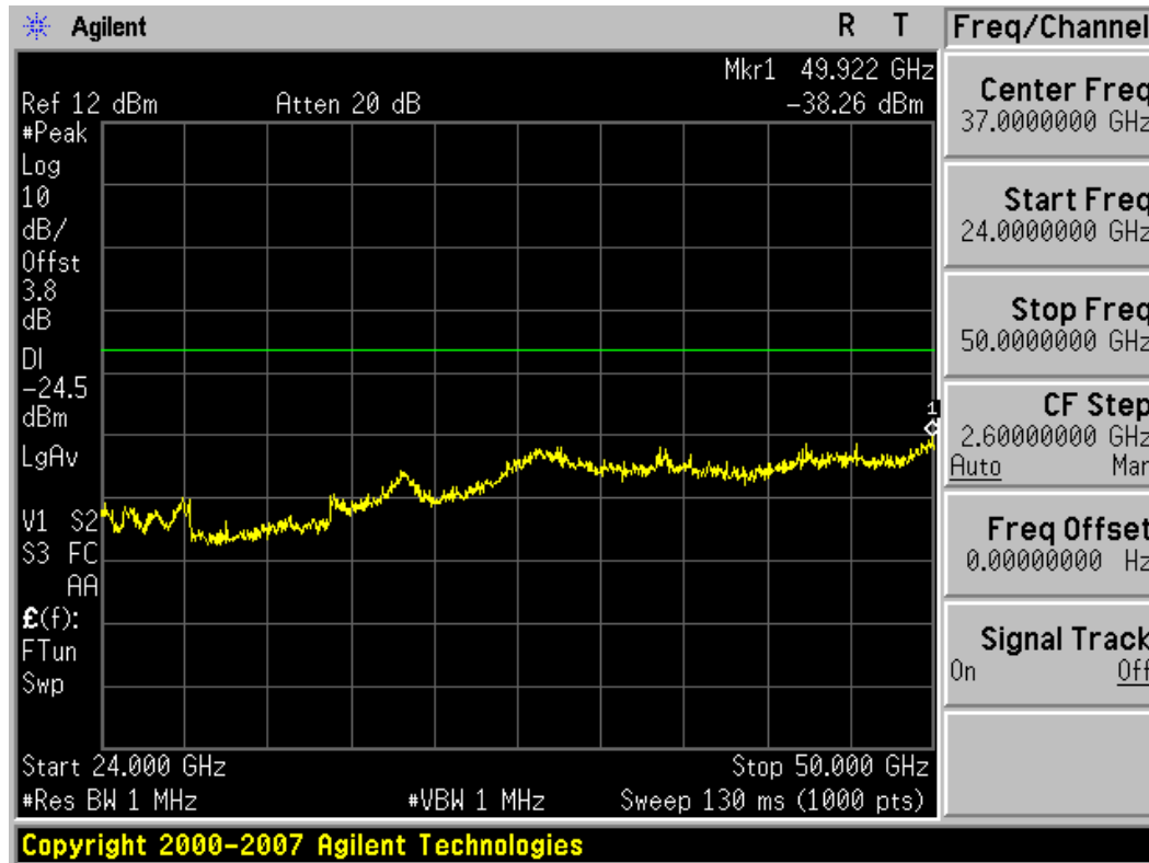
Plot 6-50. Conducted Spurious Plot (802.11a – Ch. 157)
