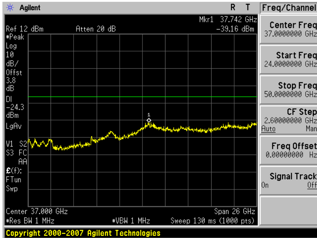
Plot 6-52. Conducted Spurious Plot (802.11a – Ch. 165)
