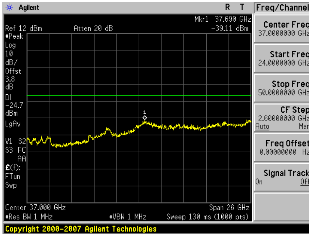
Plot 6-48. Conducted Spurious Plot (802.11a – Ch. 149)
