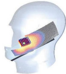
Figure 8-1 Sample SAR Area Scan
