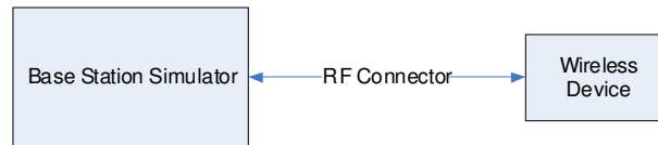
Figure 13-2 Power Measurement Setup
