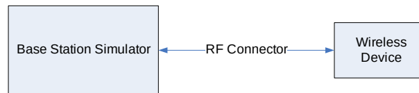
Figure 11-1 Power Measurement Setup
