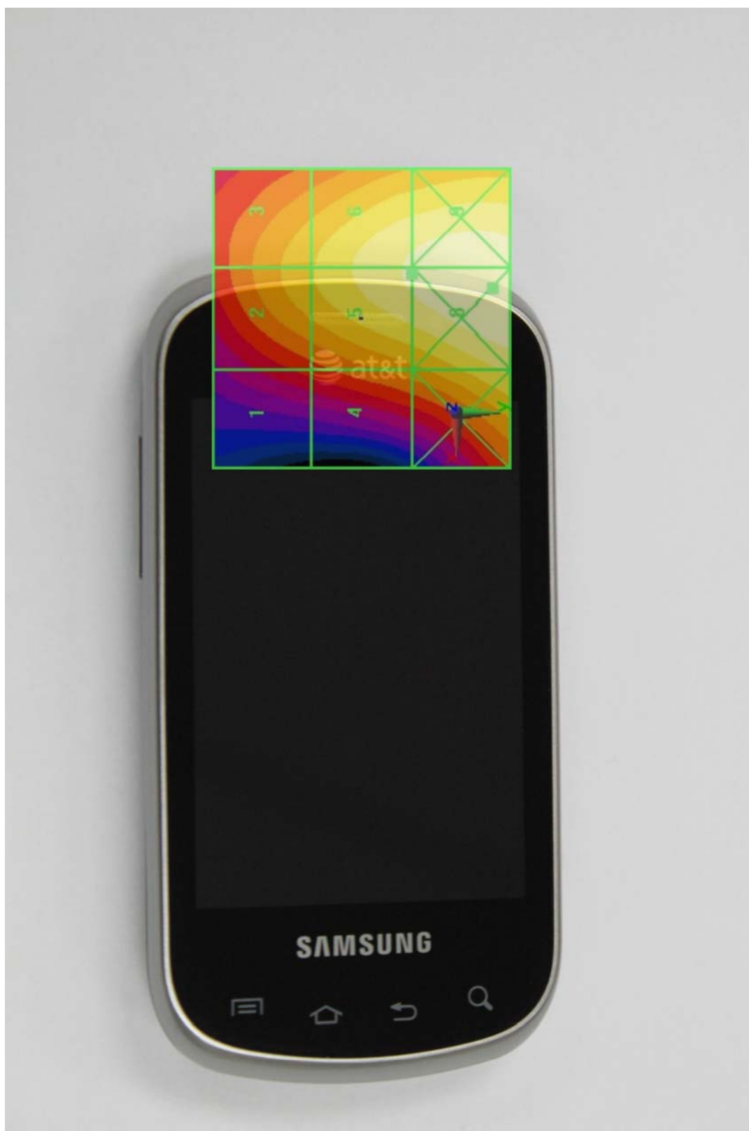
Scan Overlay with actual device(E-Field)
