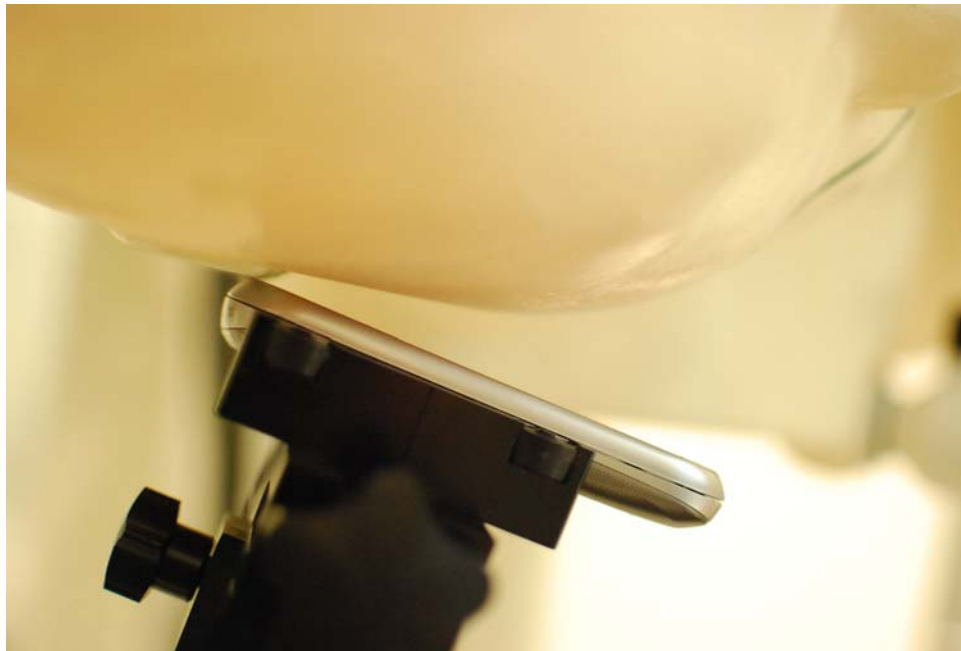
SAR Test Setup Photo 2 – Right Tilt
