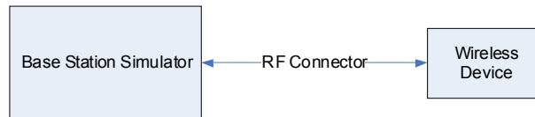
Figure 11-1 Power Measurement Setup
