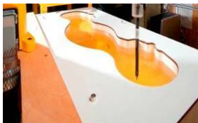
Figure 6-2 SAM Phantom with Simulating Tissue
