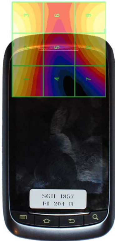
Figure 17-4 E-Field WD Scan overlay
