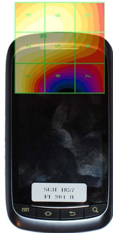
Figure 17-5 H-Field WD Scan overlay
