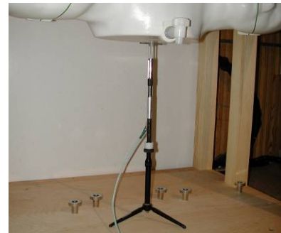
Figure 12-2 System Verification Setup Photo
