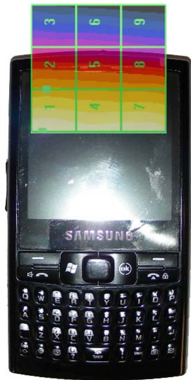
Figure 17-5 H-Field WD Scan overlay
