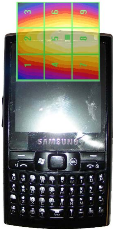
Figure 17-4 E-Field WD Scan overlay
