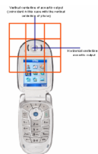
Figure 5.1 Wireless Device and Measurement Plane
