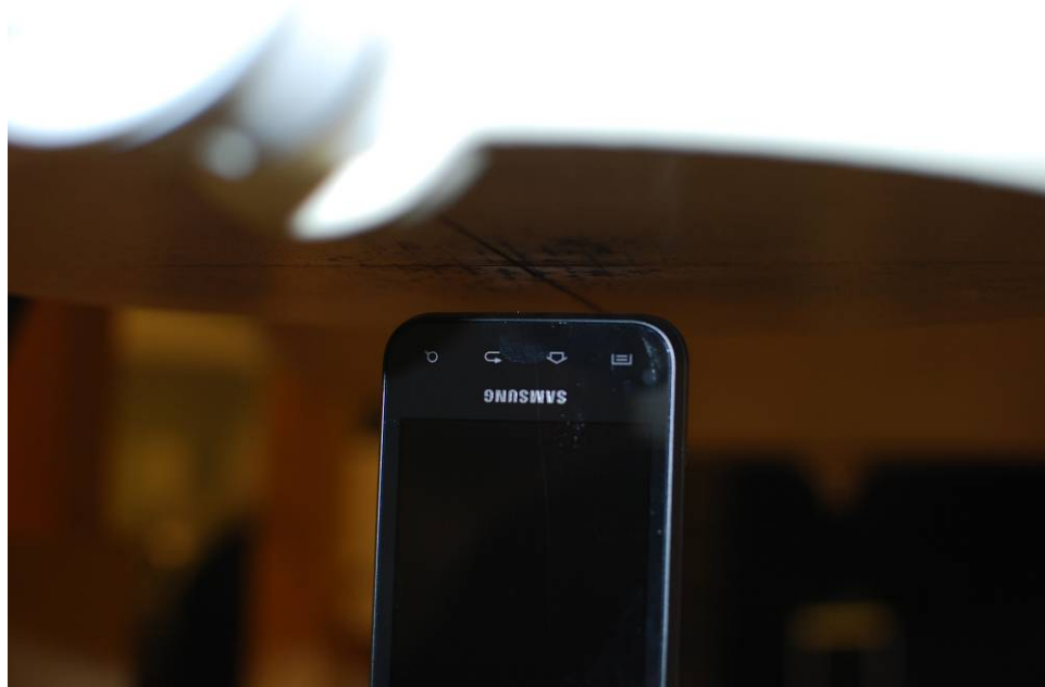
SAR Test Setup Photo 8 – Bottom at 1.0 cm
