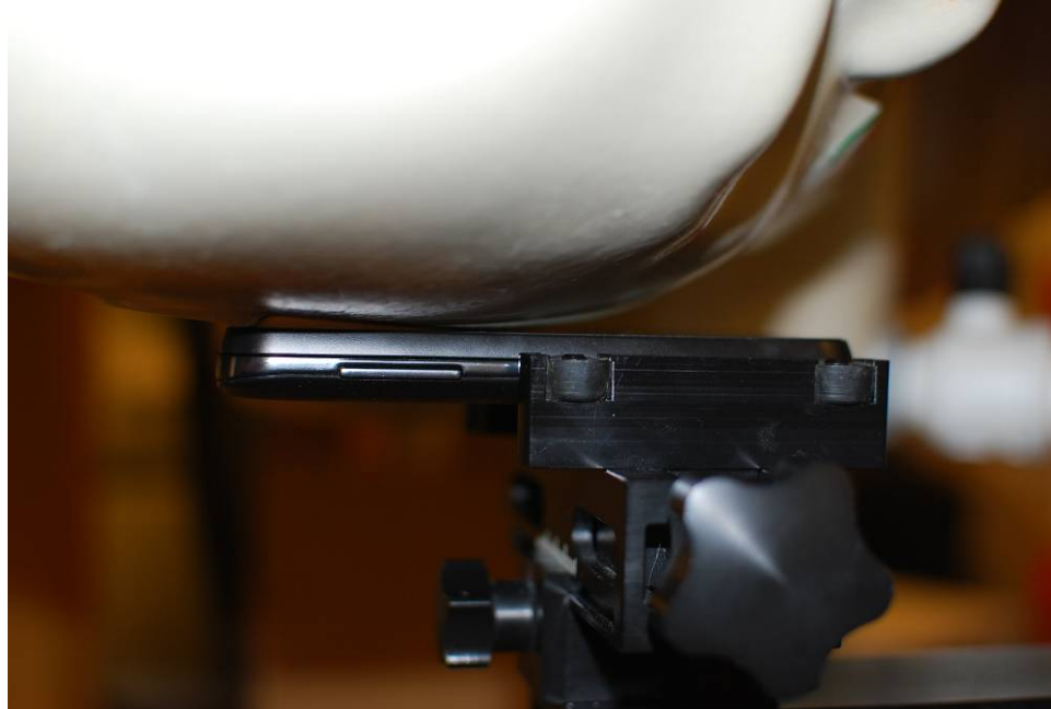
SAR Test Setup Photo 1 – Right Touch
