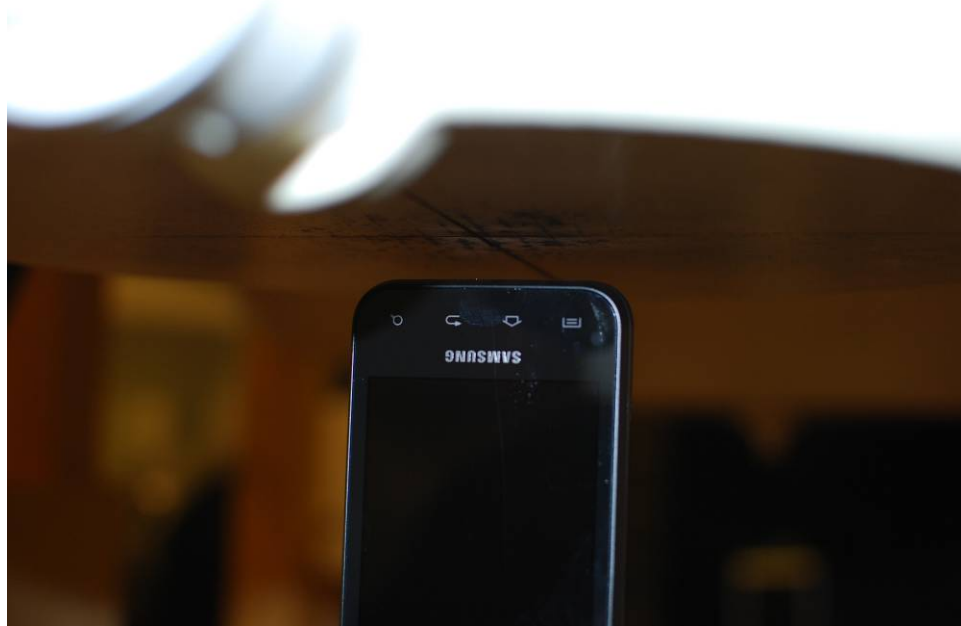
SAR Test Setup Photo 8 – Bottom at 1.0 cm
