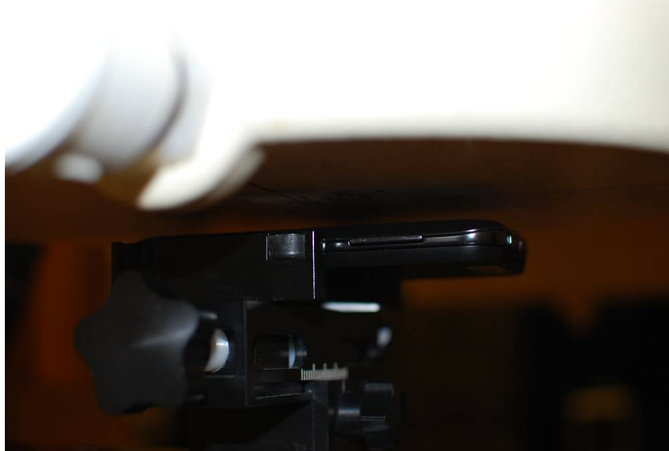
SAR Test Setup Photo 5 – Back at 1.0 cm
