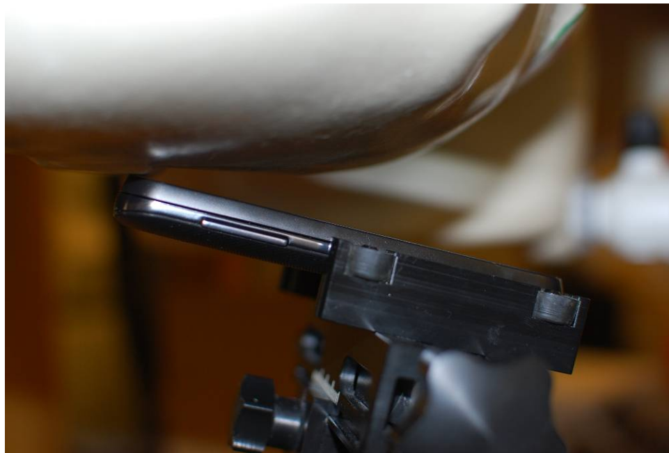
SAR Test Setup Photo 2 – Right Tilt
