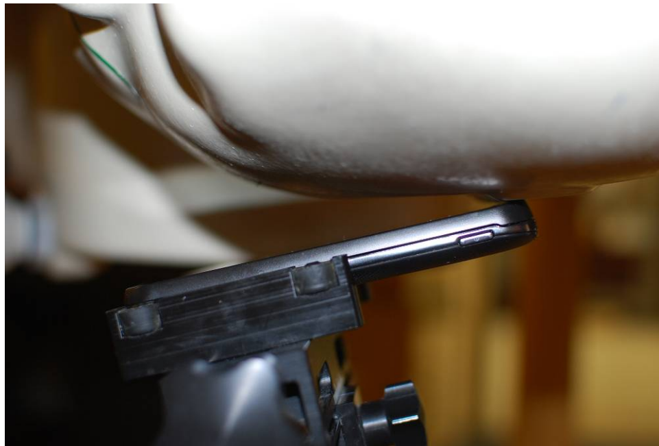
SAR Test Setup Photo 4 – Left Tilt
