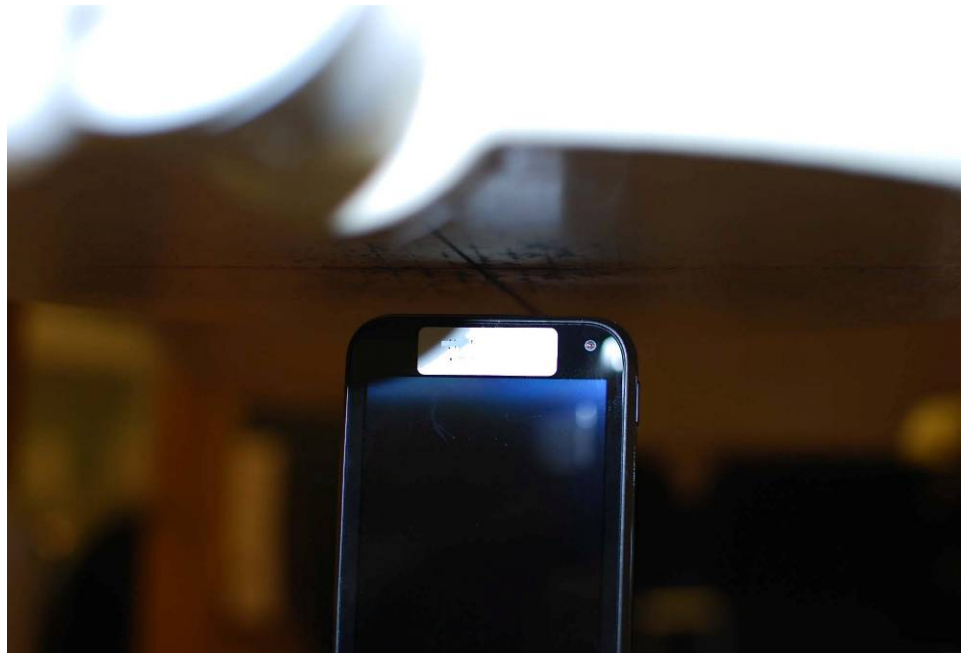
SAR Test Setup Photo 7 – Top at 1.0 cm
