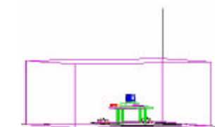
Figure 3-1. Shielded Enclosure Line-Conducted Test Facility
