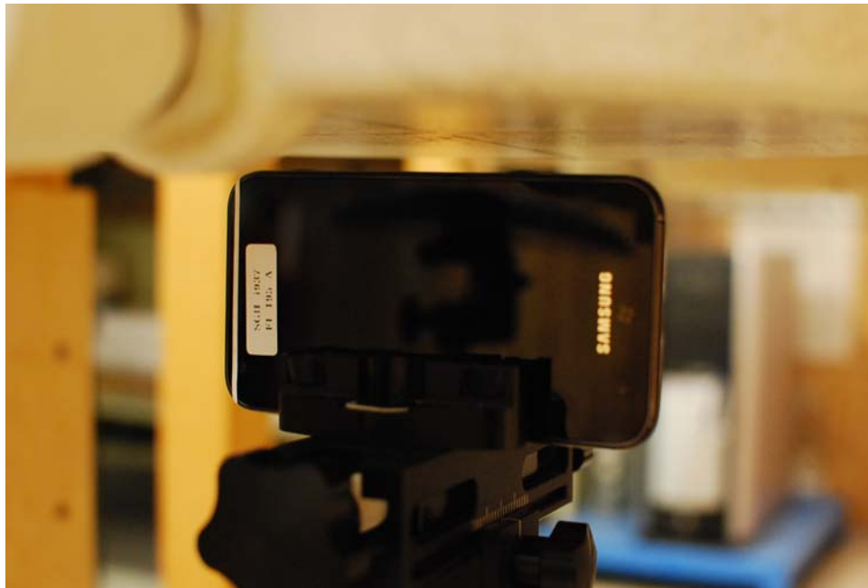
SAR Test Setup Photo 9: Right at 1.0 cm
