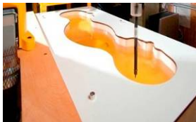
Figure 6-2 SAM Phantom with Simulating Tissue
