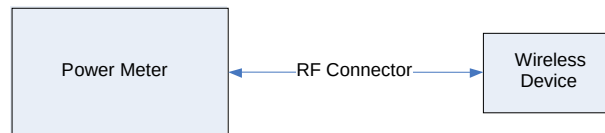
Figure 12-1 Power Measurement Setup
