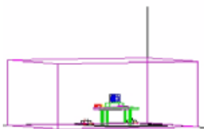
Figure 3-1. Shielded Enclosure Line-Conducted Test Facility
