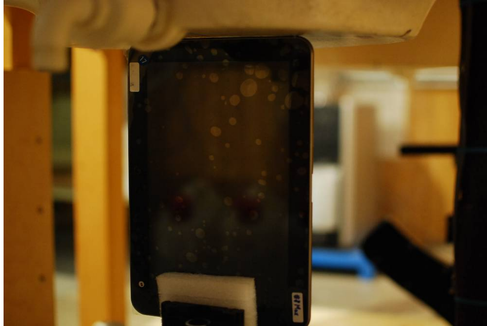
SAR Test Setup Photo 7: Left at 0.0 cm
