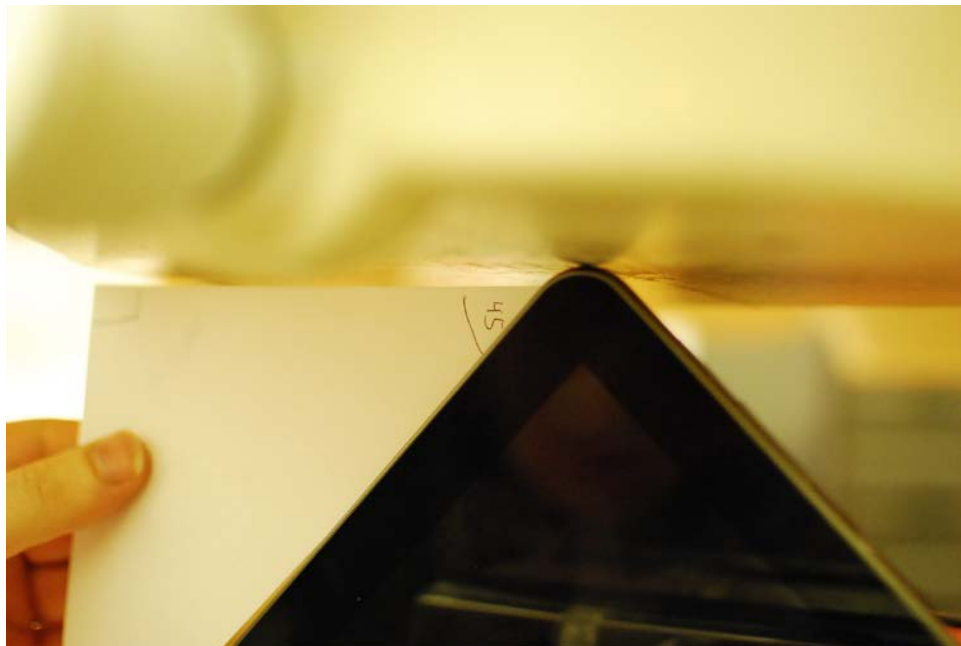
SAR Test Setup Photo 8: Vertex at 0.0 cm
