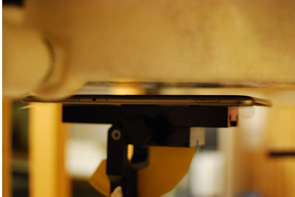
SAR Test Setup Photo 1: Back at 1.0 cm
