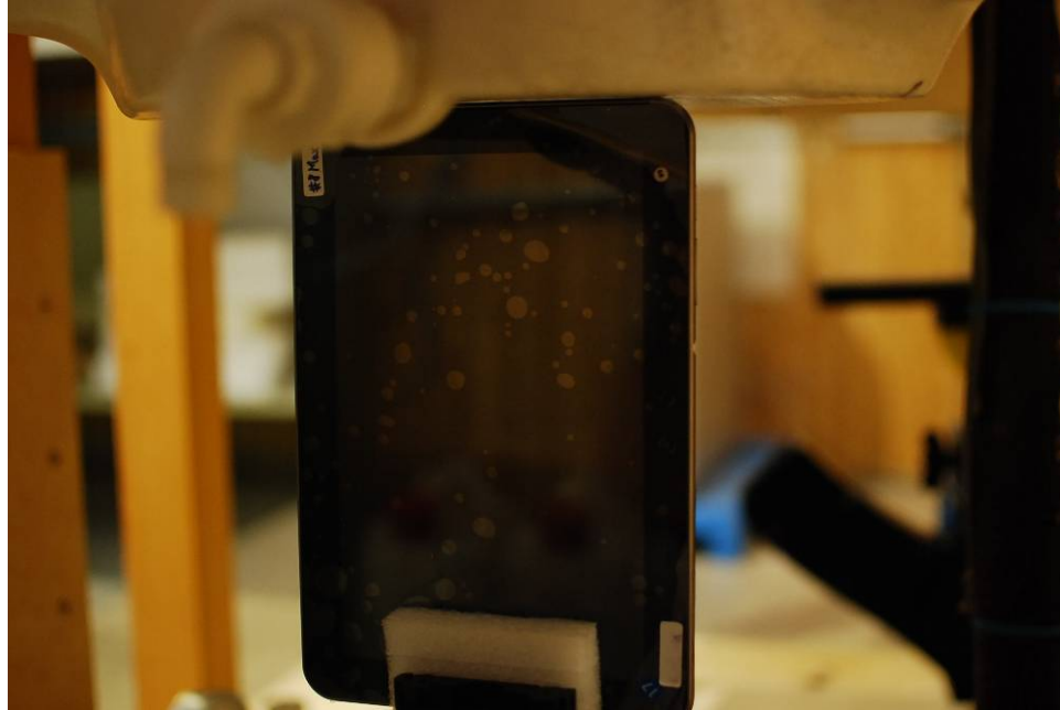
SAR Test Setup Photo 5: Right at 0.0 cm
