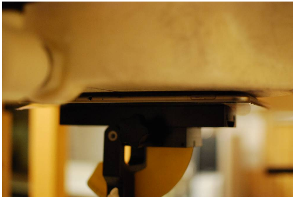
SAR Test Setup Photo 2: Back at 0.0 cm
