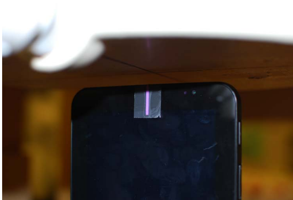
Figure 17-2 SAR Test Setup Photo 2 - Top at 0.5 cm
