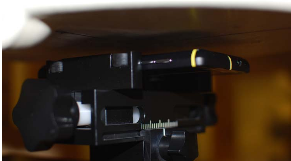
Figure 21-5 SAR Test Setup Photo 5 – Back at 1.0 cm
