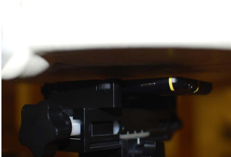
Figure 21-6 SAR Test Setup Photo 6 – Front at 1.0 cm
