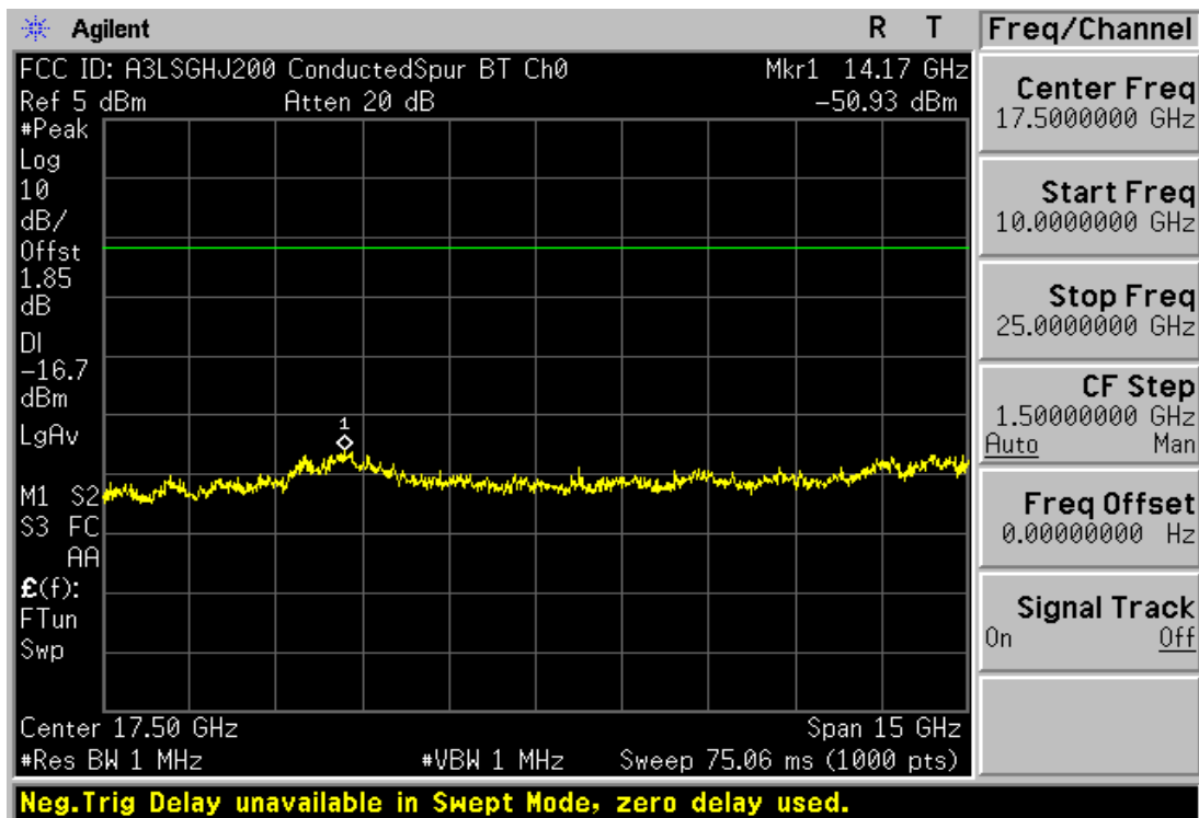
Plot 6-13. Conducted Spurious Plot (Bluetooth – Ch. 0)
