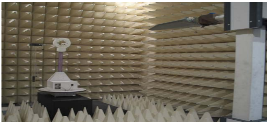
Figure2. Photograph of 3m Fully-Anechoic Chamber
