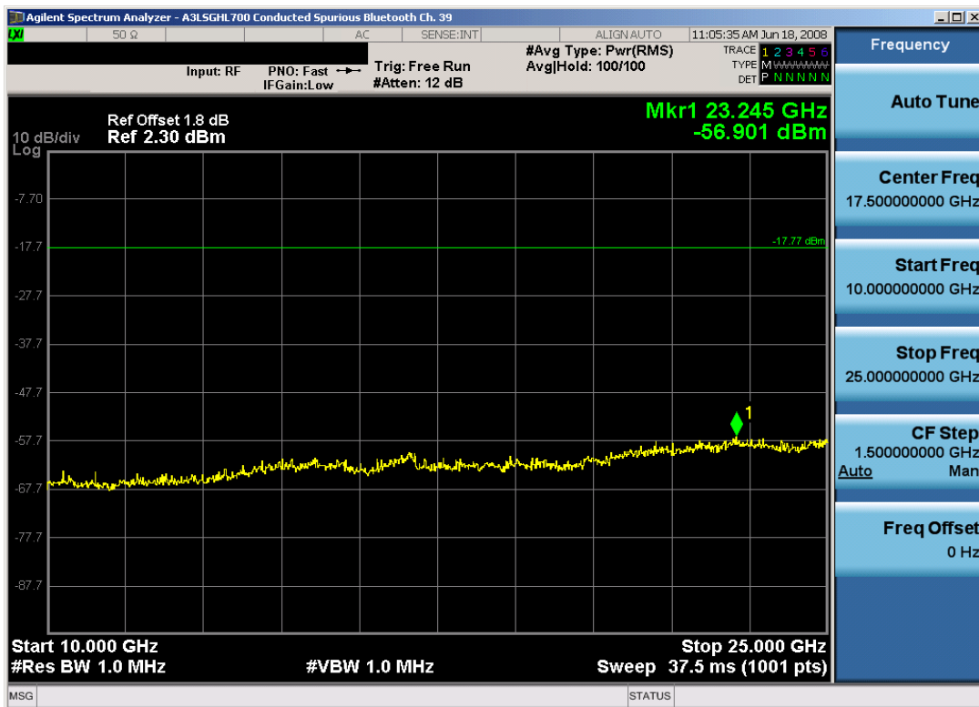
Plot 6-15. Conducted Spurious Plot (Bluetooth – Ch. 39)
