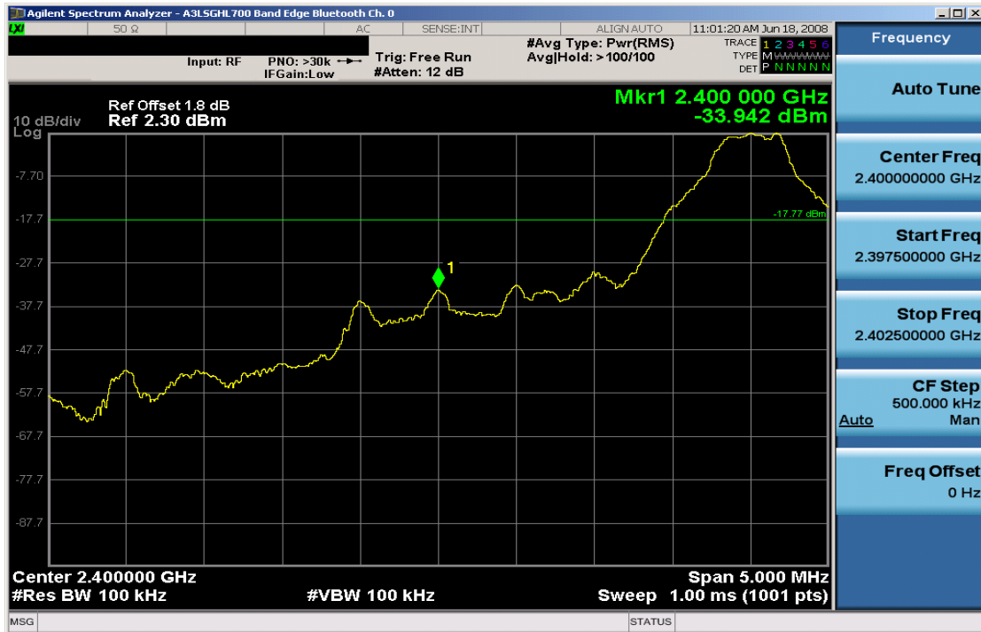
Plot 6-4. Band Edge Plot (Bluetooth – Ch. 0)
