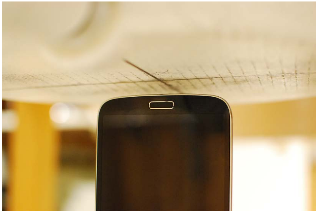
SAR Test Setup Photo 8: Bottom at 1.0 cm
