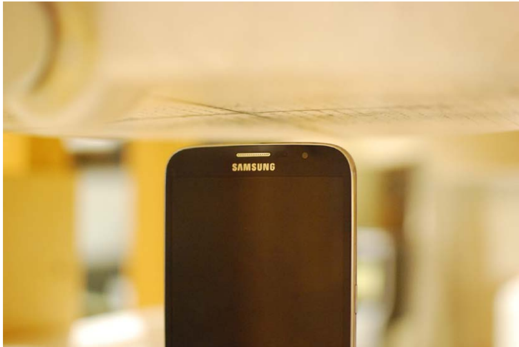
SAR Test Setup Photo 7: Top at 1.0 cm
