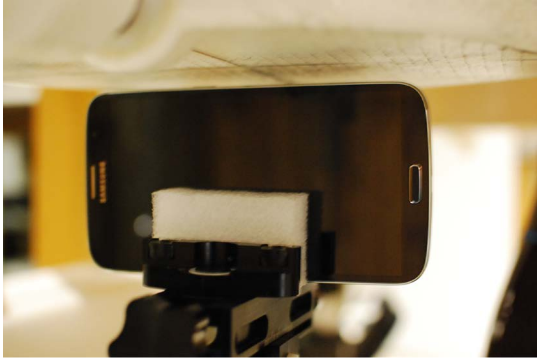
SAR Test Setup Photo 9: Right at 1.0 cm
