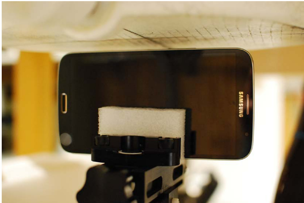
SAR Test Setup Photo 10: Left at 1.0 cm
