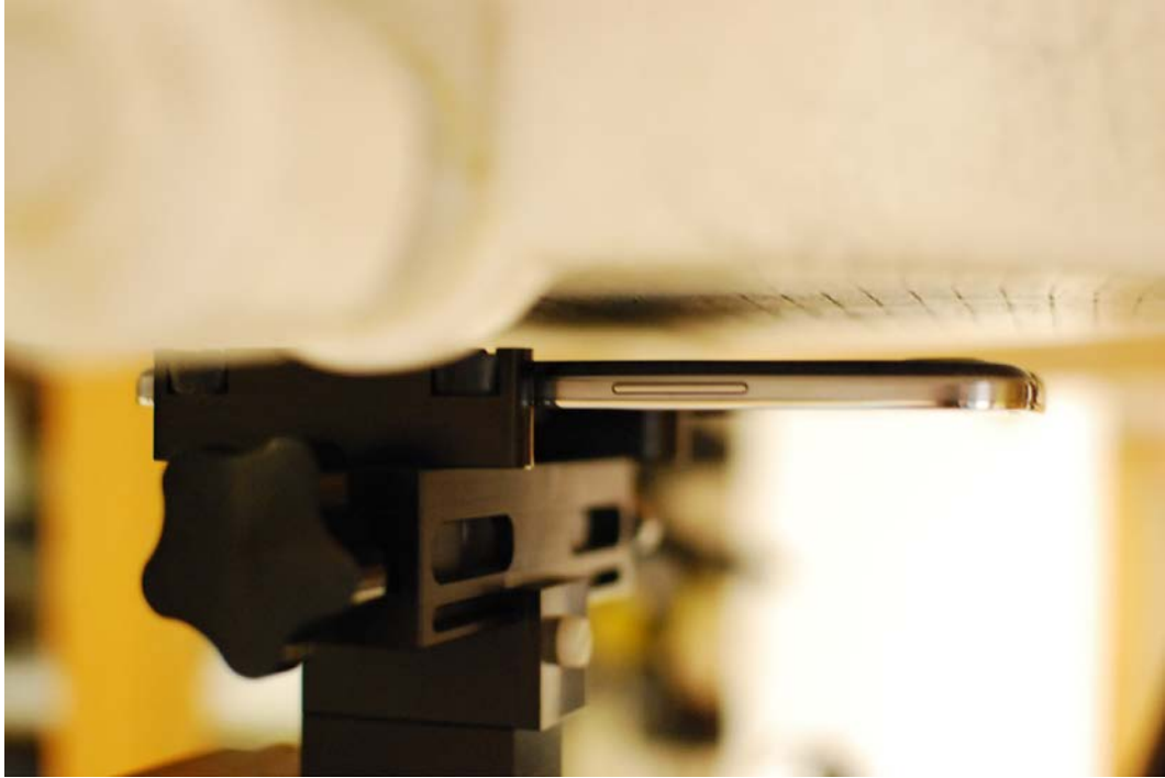
SAR Test Setup Photo 5: Back at 1.0 cm
