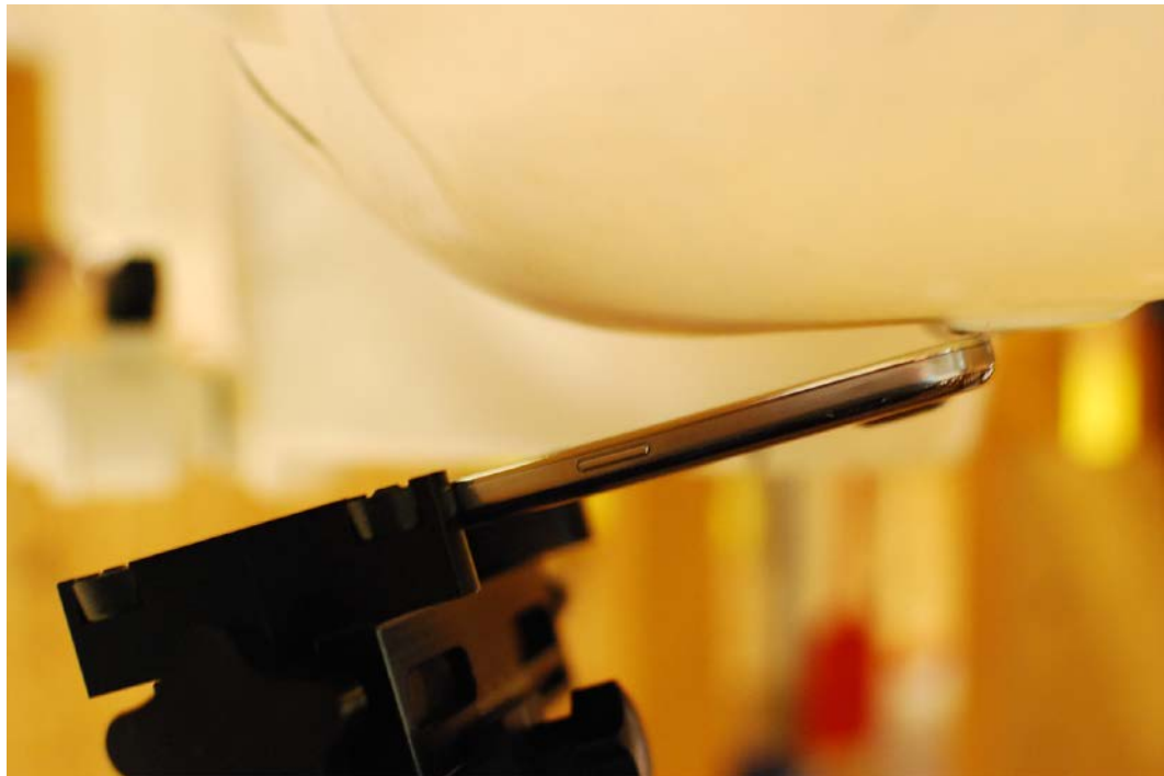
SAR Test Setup Photo 4: Left Tilt
