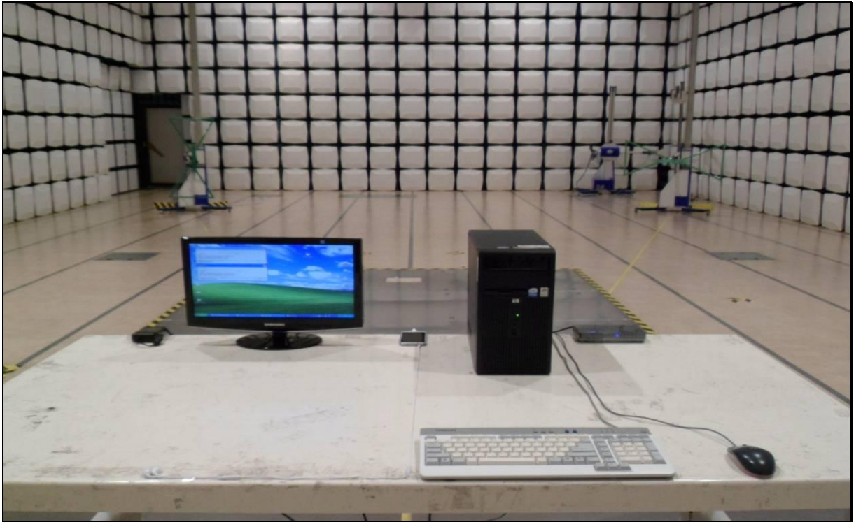
[ Radiated Disturbance for Below 1 GHz – Front ]
