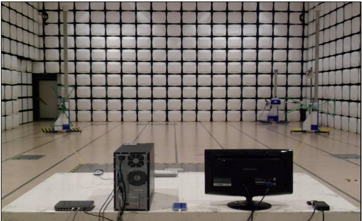
[ Radiated Disturbance for Below 1 GHz – Rear ]
