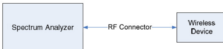
Figure 6-1. Test Instrument & Measurement Setup
